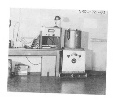
Fig. 2.8 4-pi Ionization Chamber
