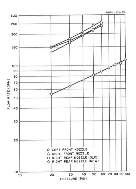
Fig. 2.3 Calibration of Nozzle Flow Rates at Pressures of Interest
