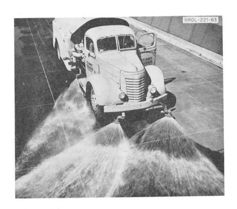
Fig. 2.6 Three-nozzle Operation at Settings Used for Evaluation Tests.
