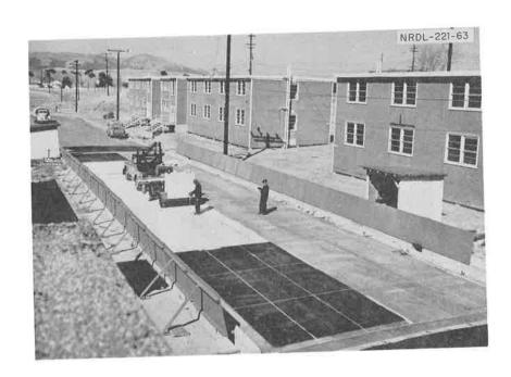
Fig. 2.9 Measuring Radiation Intensity of Synthetic Fallout with Scintillation Counter and Hand-held Radiac.
