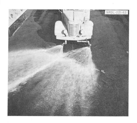
Fig. 2.5 Front Nozzle Operation Showing Protractor Bar Used to Obtain Proper Nozzle Orientation. Protractor points occur every 10 degrees.
