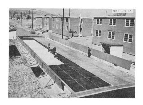
Fig. 2.7 Dispersal of Synthetic Fallout on Test Area by Hand-pulled Garden Spreader.
