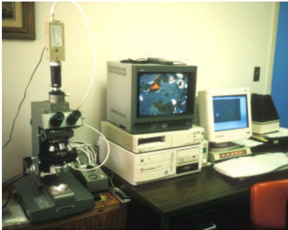
Polarized light microscope to identify sources and characteristics of stormwater particulates
