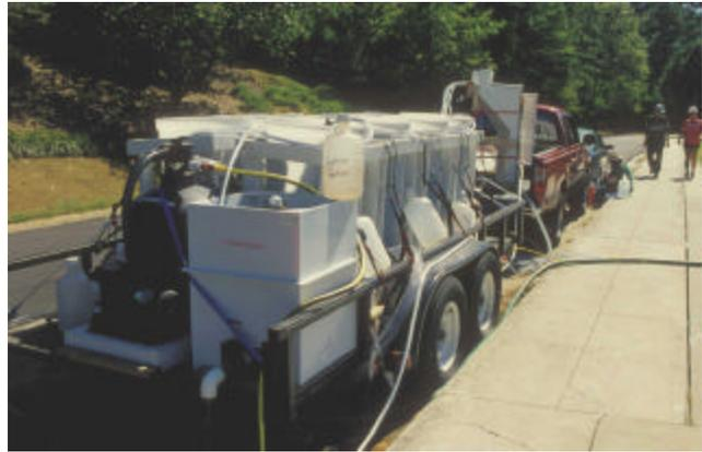
Pilot-scale filtration setup for post-sedimentation treatment tests
