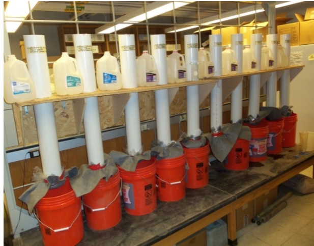
Figure X.4 Laboratory column setup for infiltration measurements.
