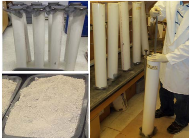
Figure X.3 Lab column construction for infiltration tests (left to right): bottom of the columns secured with a fiberglass window screen (upper left), North Carolina bioretention media (lower left), and media compaction
