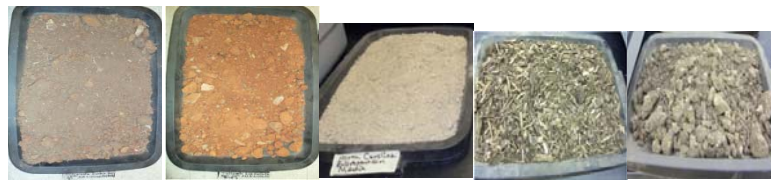
Figure X.1 Media (from left to right): Tuscaloosa surface soil, Tuscaloosa subsurface soil, North Carolina biofilter media, Kansas City biofilter media from test sites 1 and 2.
