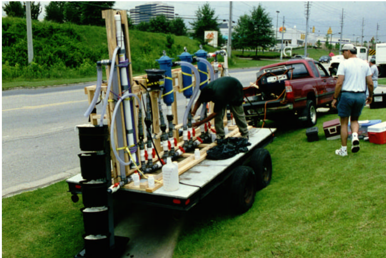
Figure 6.35. Pilot-scale treatment train showing configuration of treatment processes and sample collection locations.
