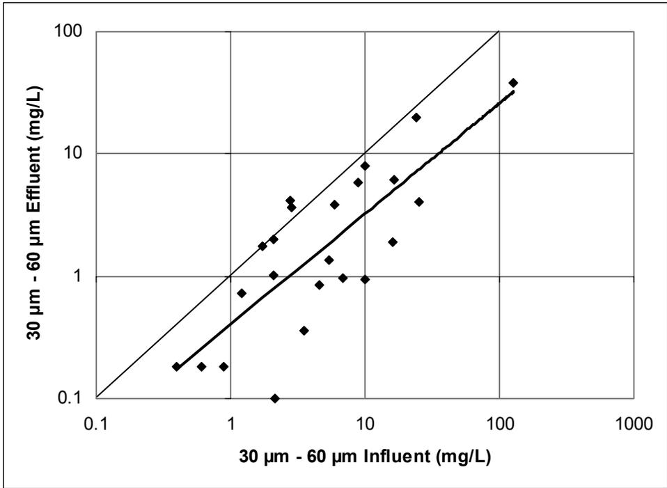
Scatterplot of observed influent and effluent 30 to 60 µm particle size concentrations.
