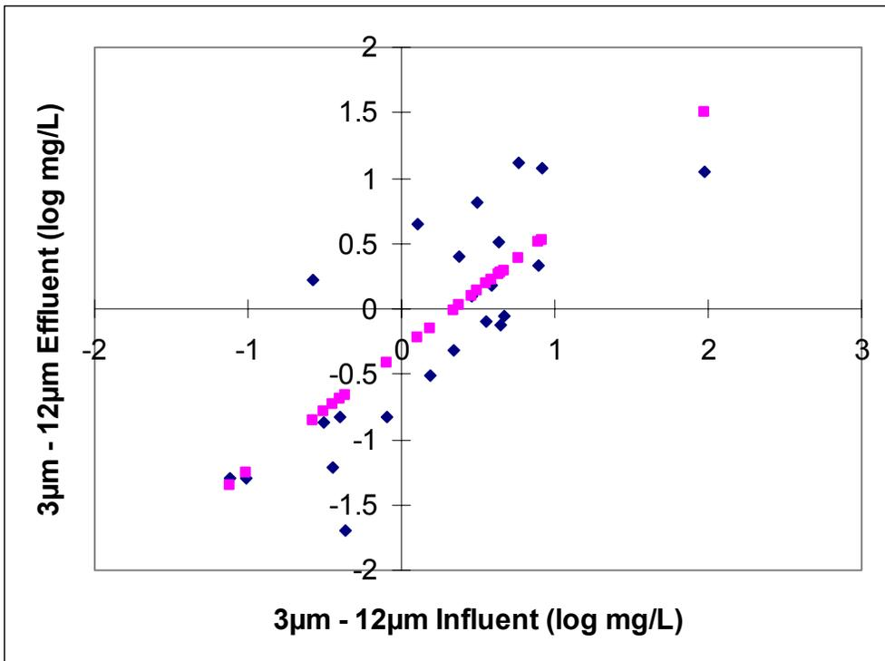
Fitted equation and data points for influent and effluent 3 to 12 µm particle size.
