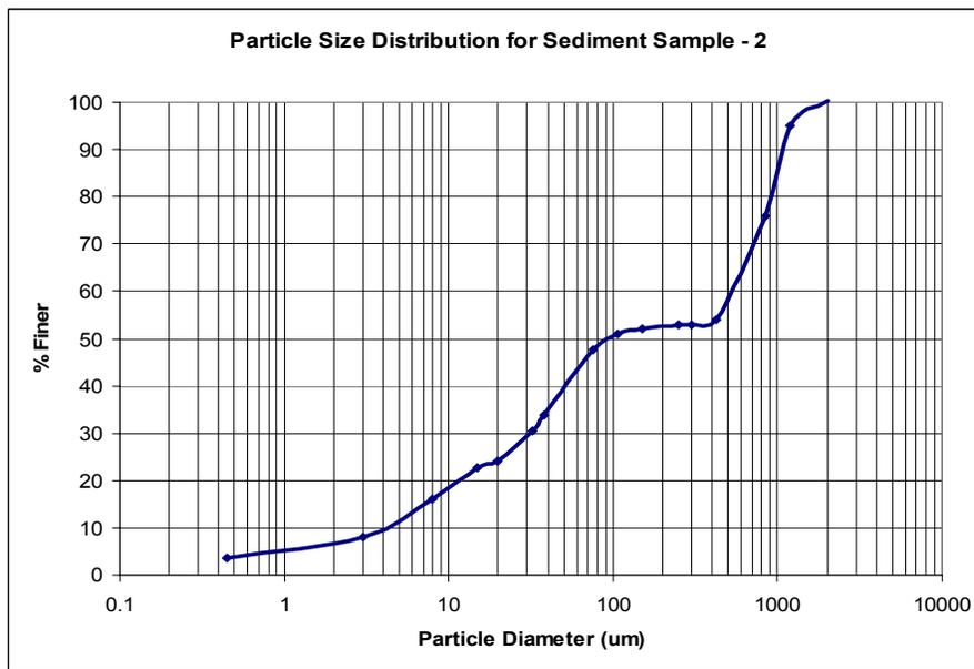
Figure 4-4: PSD curve for test sediment sample 2.
