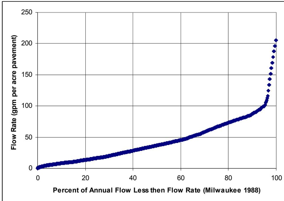
Figure 5-20: Treatment flow rates needed for Milwaukee, WI.
