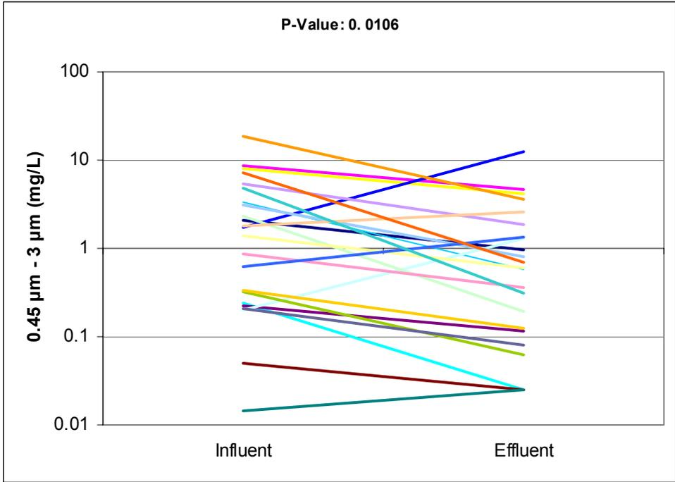
Paired influent and effluent 0.45 to 3 µm particle size concentrations.
