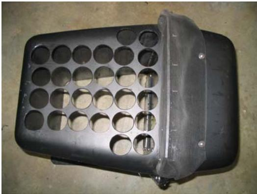
**Figure 2-2: Bottom of Up-Flo™ Filter prototype shown without angled screen - at left, the large holes serve as an inlet to the filtration chamber and at right, a finer screen sits over weep hole tubes for blockage protection.**
