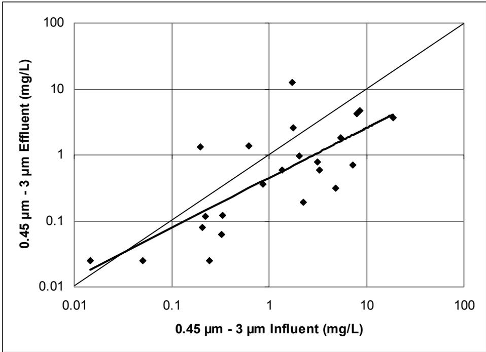
Scatterplot of observed influent and effluent 0.45 to 3 µm particle size concentrations.
