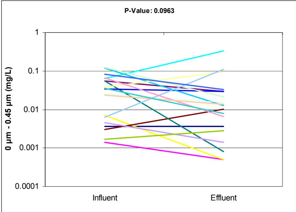
Paired influent and effluent 0 to 0.45 µm particle size concentrations.
