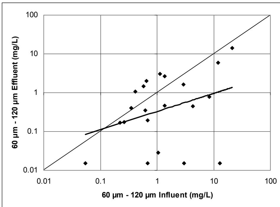
Scatterplot of observed influent and effluent 60 to 120  $\mu$ m particle size concentrations.
