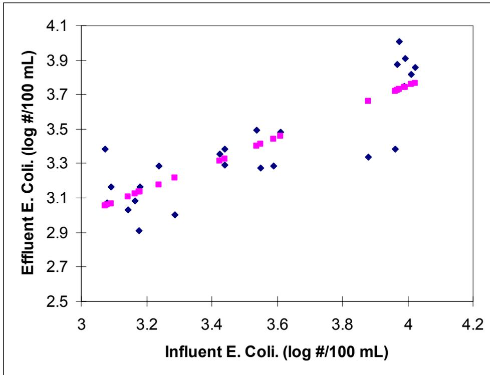
Fitted equation and data points for influent and effluent E. Coli.
