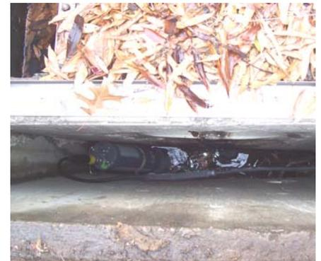
**Figure 4-26: Sonde in the effluent chamber.**
