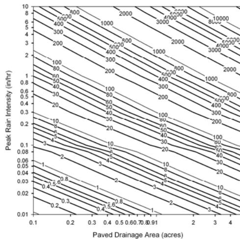
Figure 3-9: Calculated peak runoff rates (gallons/minute) for different peak rain intensities and drainage areas for paved areas.
