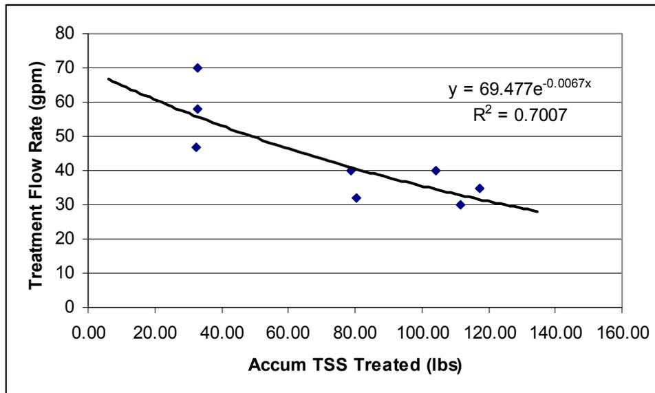
Figure 4-33: Up-Flo™ Filter treatment rate with suspended solids treated.
