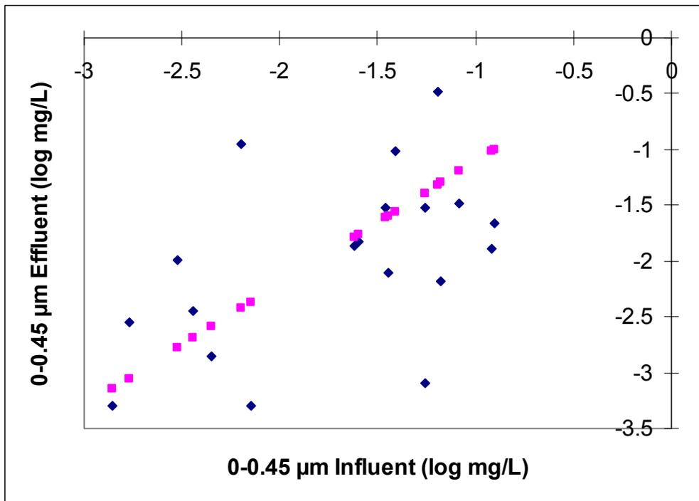
Fitted equation and data points for influent and effluent 0 to 0.45 µm particle size.
