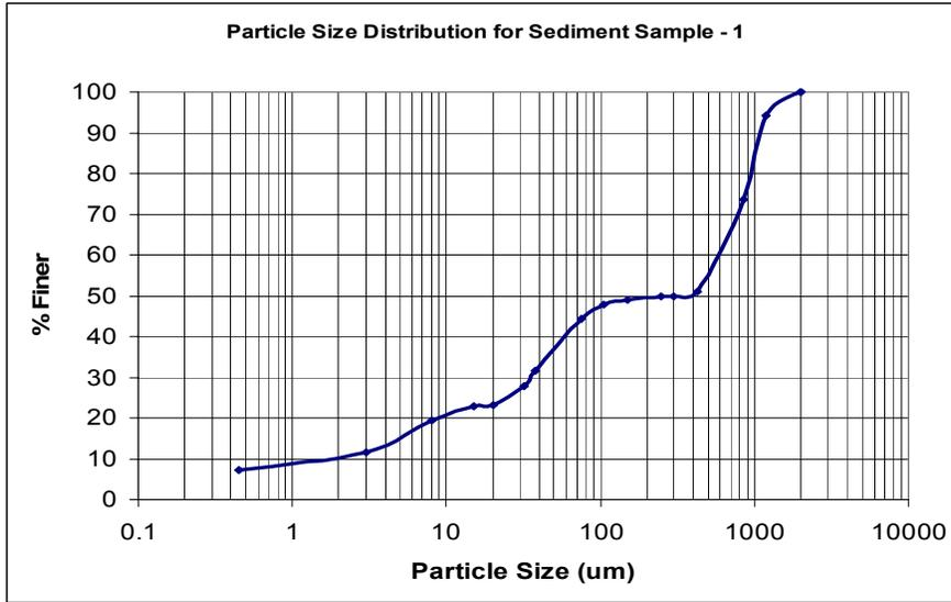
Figure 4-3: PSD curve for test sediment sample 1.
