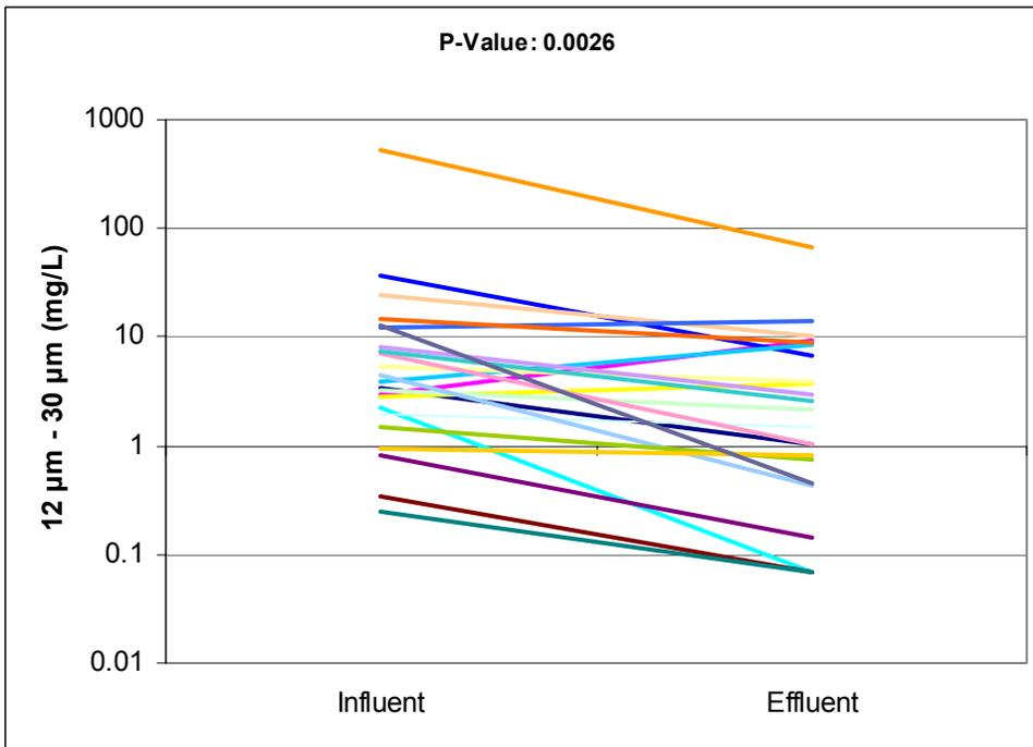
Paired influent and effluent 12 µm to 30 µm particle size concentrations.
