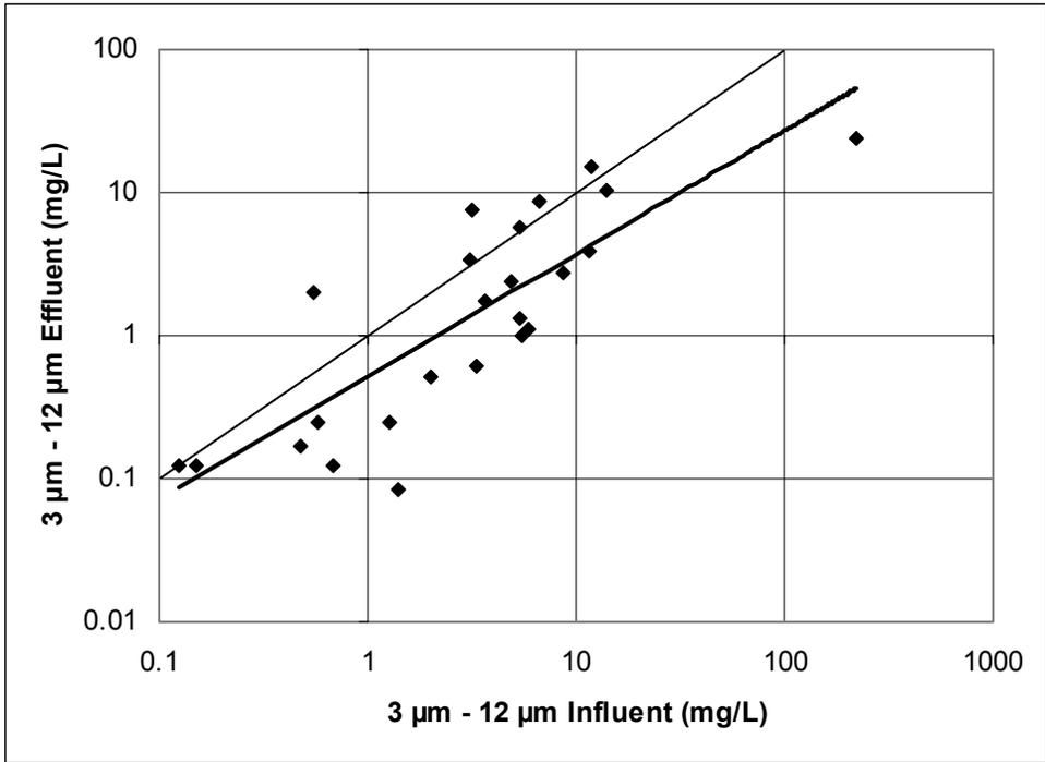
Scatterplot of observed influent and effluent 3 to 12 µm particle size concentrations.
