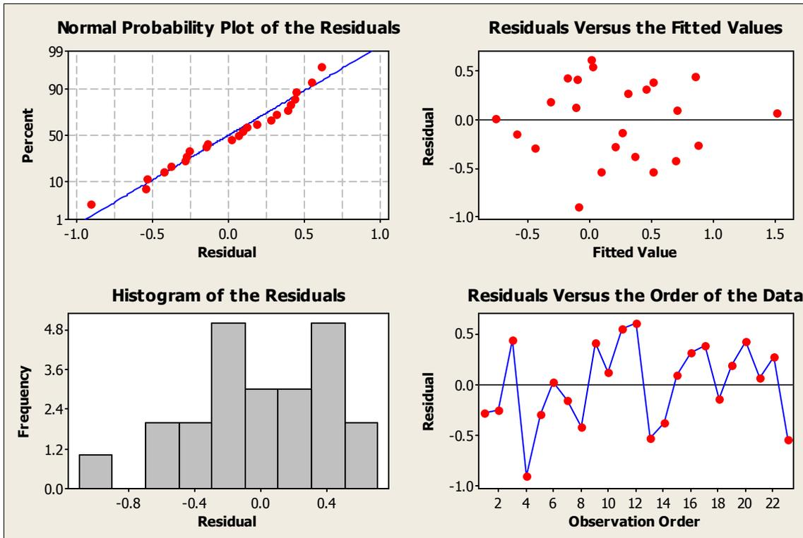
Residual analyses of fitted equation for 30 to 60  $\mu$ m particle size influent vs. effluent.
