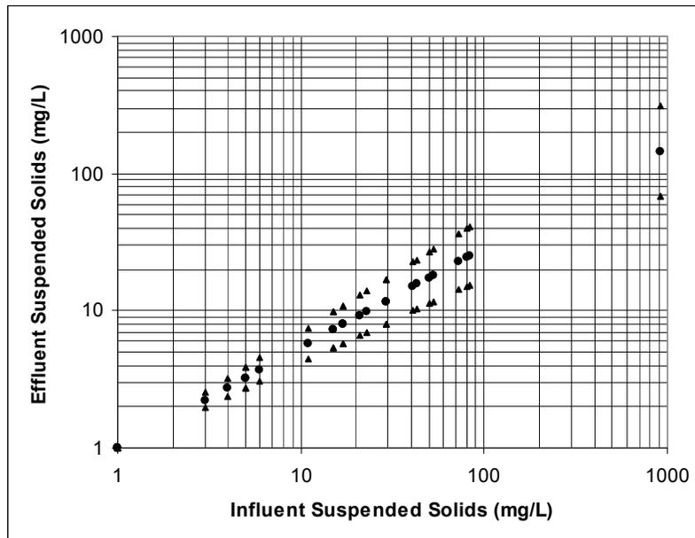
Figure 5-9: Predicted effluent concentrations for different influent concentrations, with 95% confidence limits.
