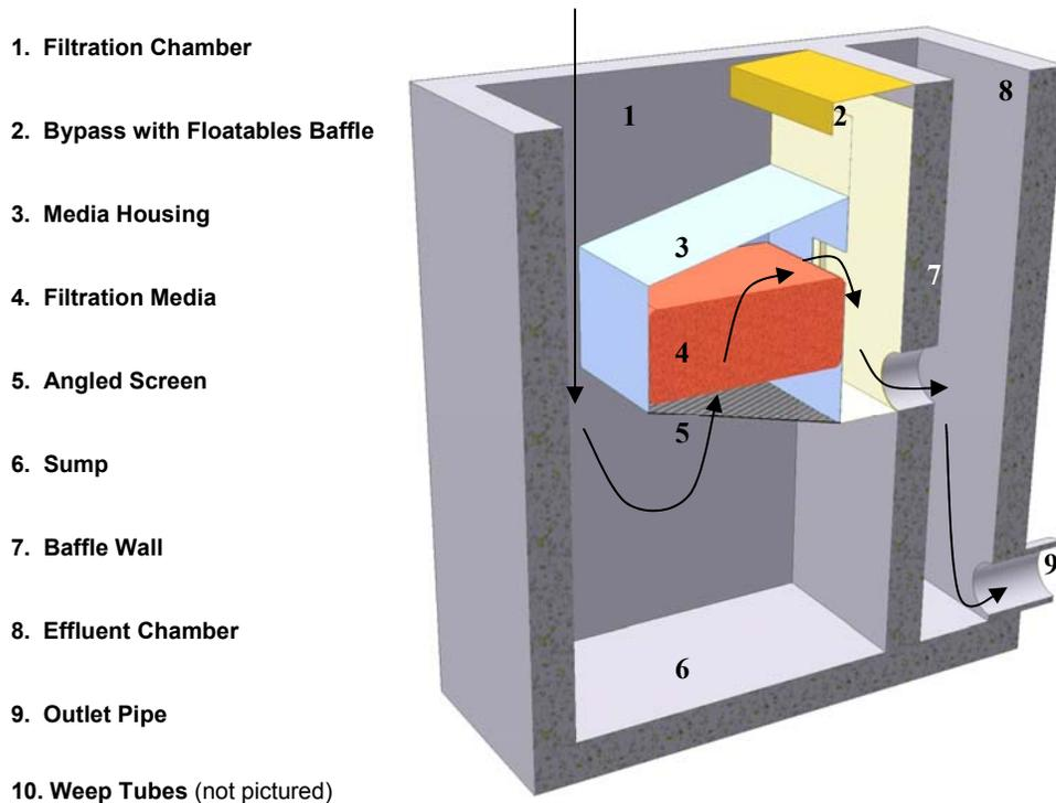
**Figure 2-1: Schematic of Up-Flo™ Filter prototype.**
