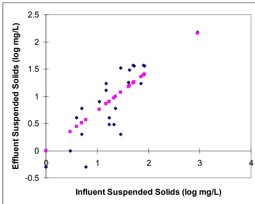
**Figure 5-7: Fitted equation and data points for influent and effluent suspended solids.**
