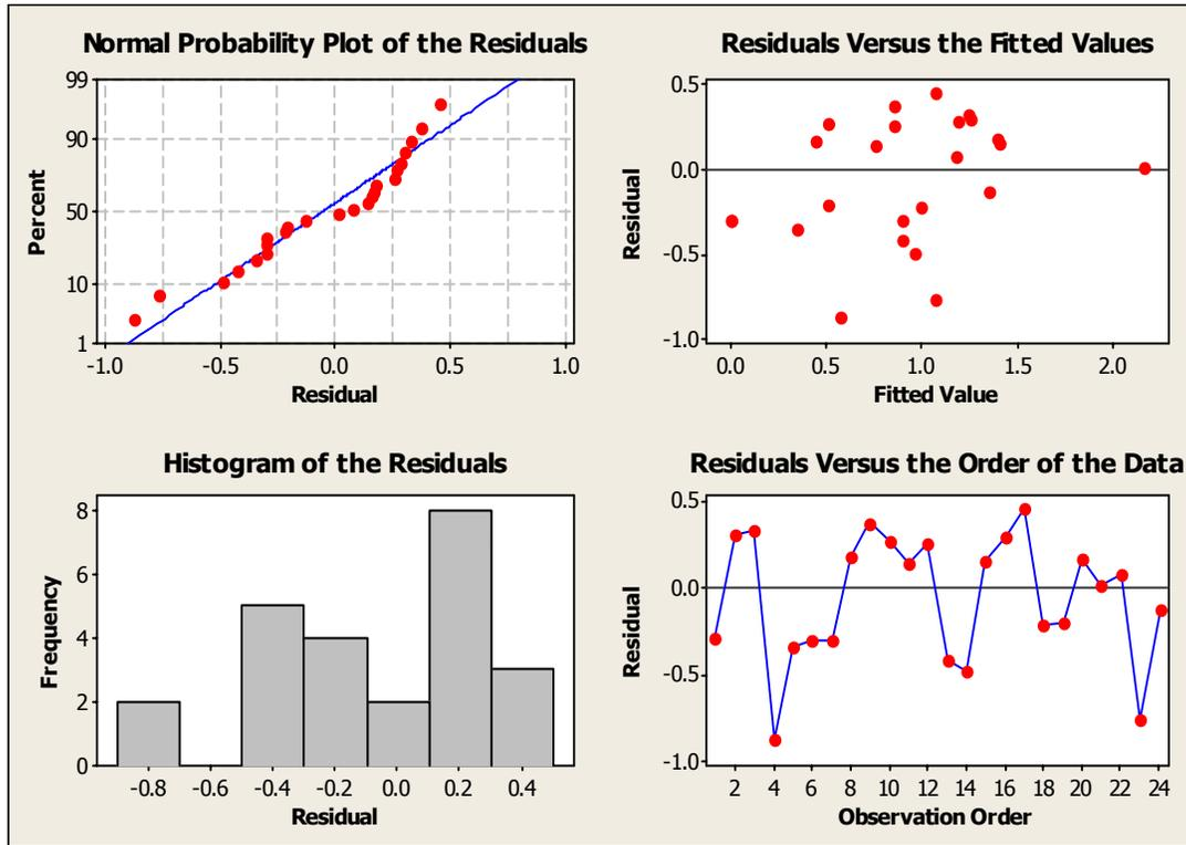
Figure 5-8: Residual analyses of fitted equation for suspended solids influent vs. effluent.
