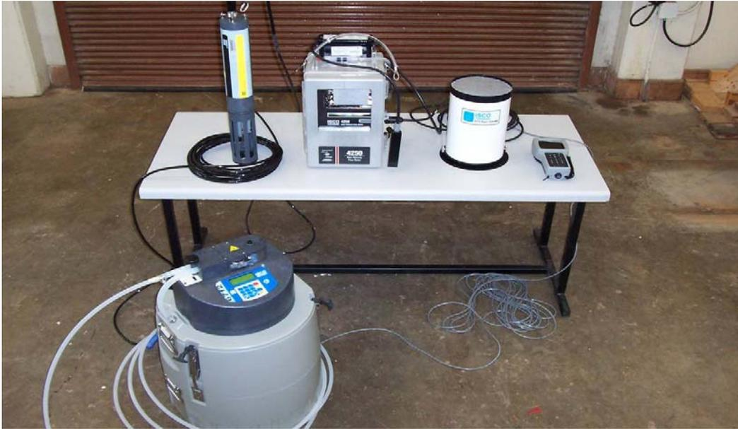
Figure 4-15: From bottom left to right 1) ISCO 6712 automatic sampler 2) YSI 6600 Sonde 3) ISCO 4250 Flow Meter 4) ISCO 674 Tipping bucket rain gauge 5) YSI Sonde data logger.
