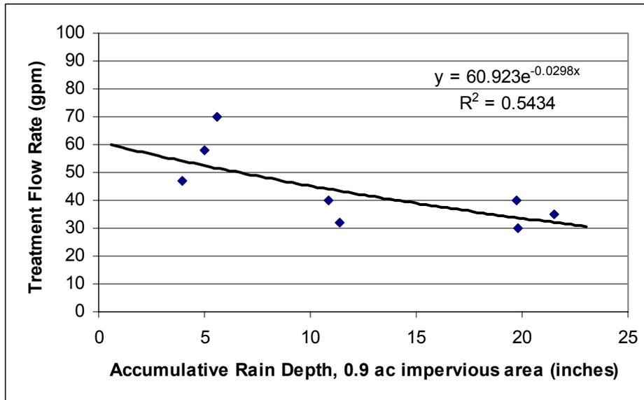
Figure 4-31: Up-Flo™ Filter treatment rate with rain depth.
