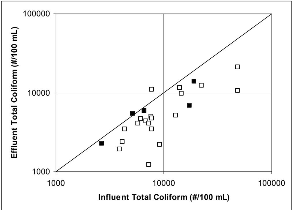
Scatterplot of observed influent and effluent total coliforms concentrations (filled symbols are events that had minor filter bypasses).
