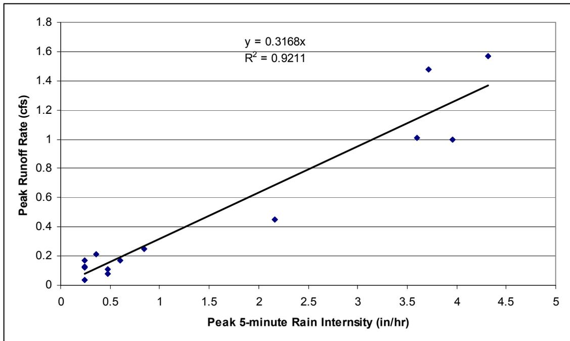
Figure 4-30: Peak 5-minute rain intensities and peak runoff rates observed.
