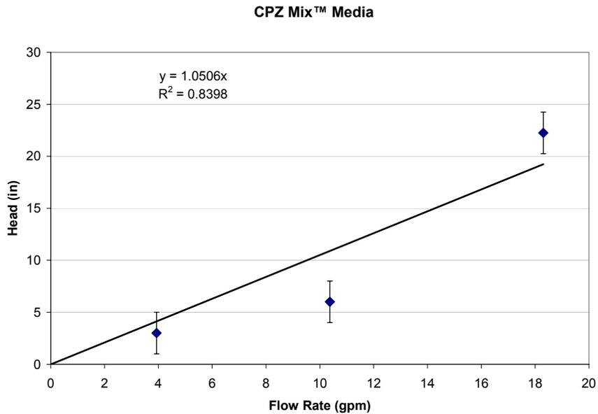
**Figure 4-2: Flow vs. head graph for mixed media**
