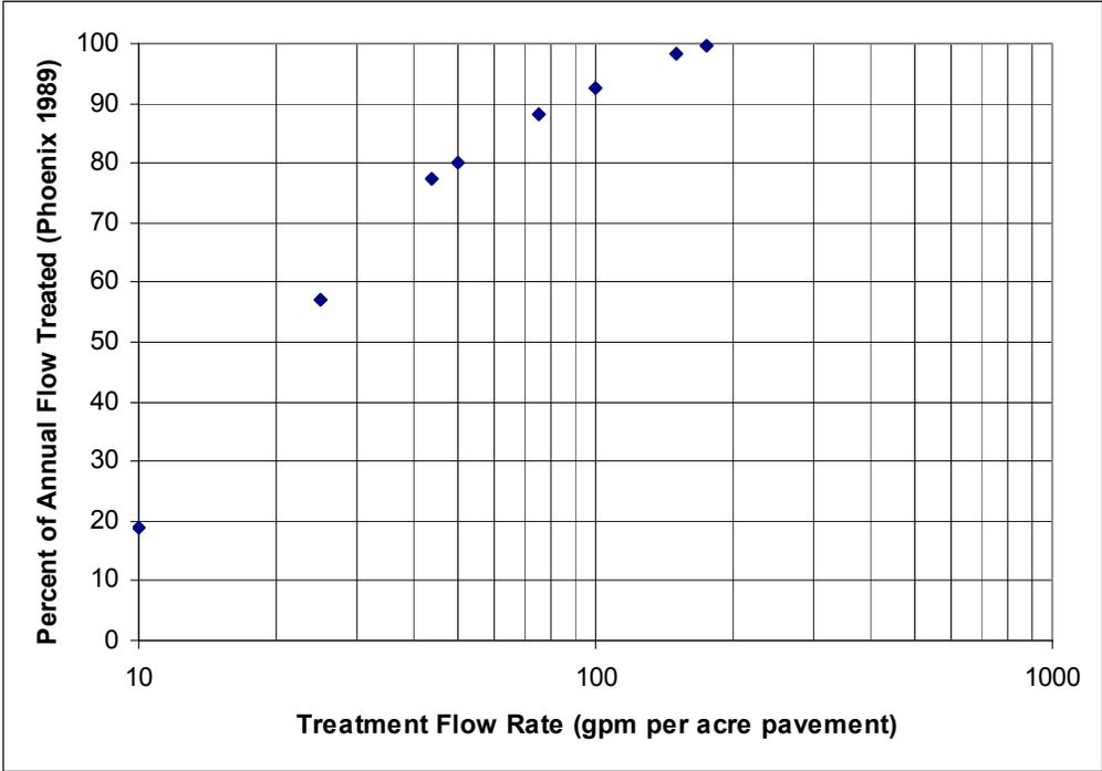
Figure 5-15: Treatment flow rates needed for Phoenix, AZ.
