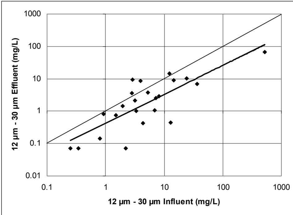
Scatterplot of observed influent and effluent 12 to 30 µm particle size concentrations.
