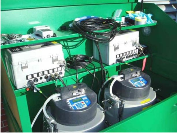
Figure 4-18: Samplers and flow meters in sampling shelter.
