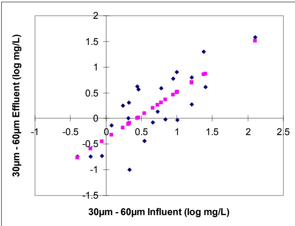
Fitted equation and data points for influent and effluent 30 to 60 µm particle size.
