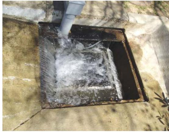
300 gpm showing overflow bypass
