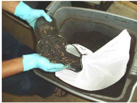
Figure 2-7: Filter bag being filled with CPZ Mix™
