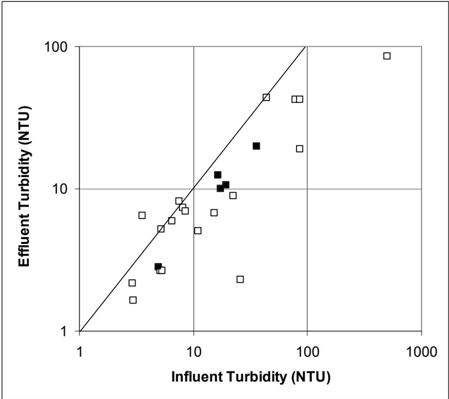
Scatterplot of observed influent and effluent turbidity concentrations (filled symbols are events that had minor filter bypasses).
