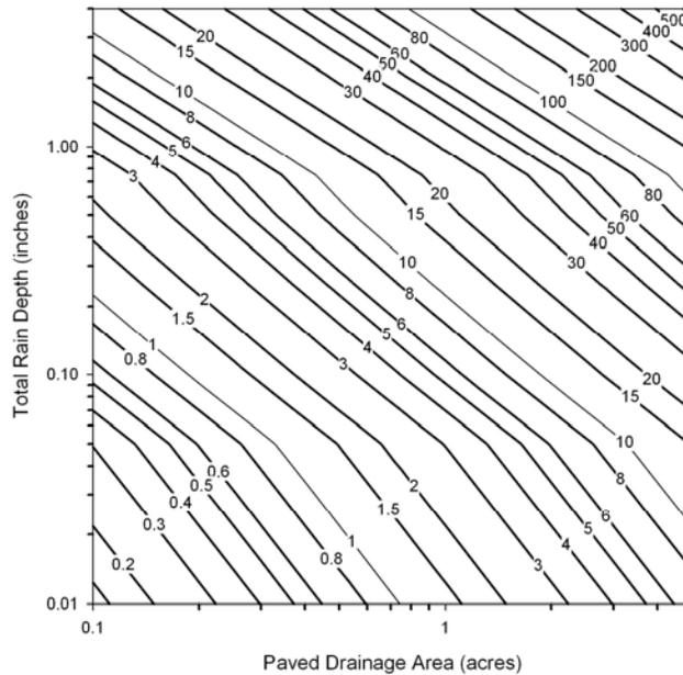
**Figure 3-10: Average runoff rates (gallons/minute) for different total event rain depths and paved drainage areas.**
