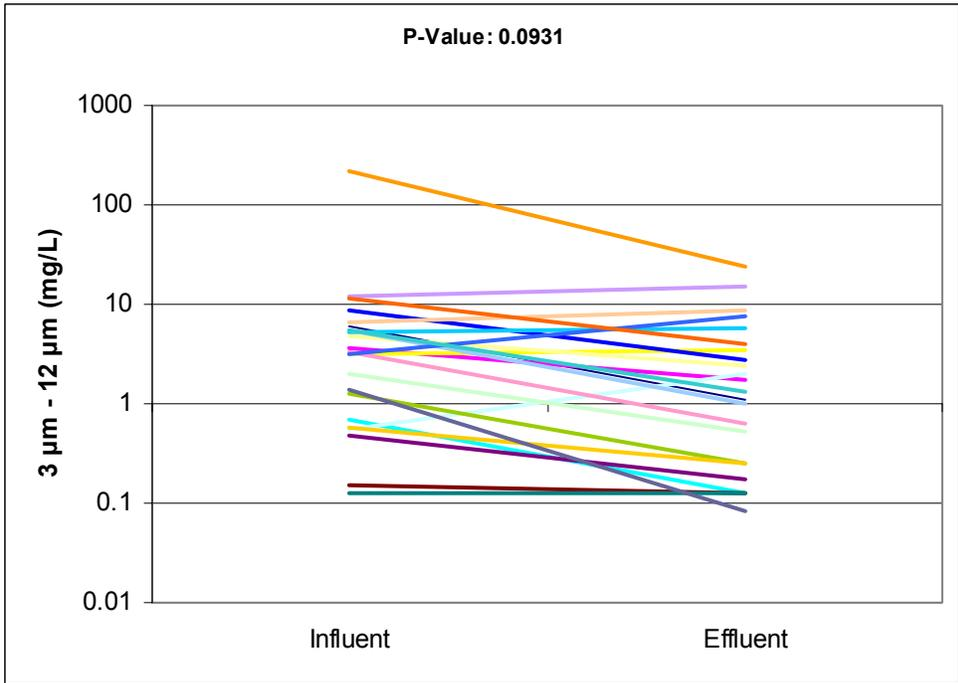
Paired influent and effluent 3 µm to 12 µm particle size concentrations.
