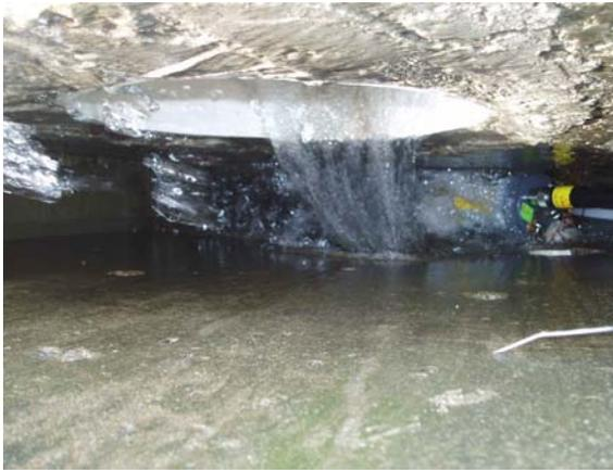
Effluent pouring onto sonde and sample intake
