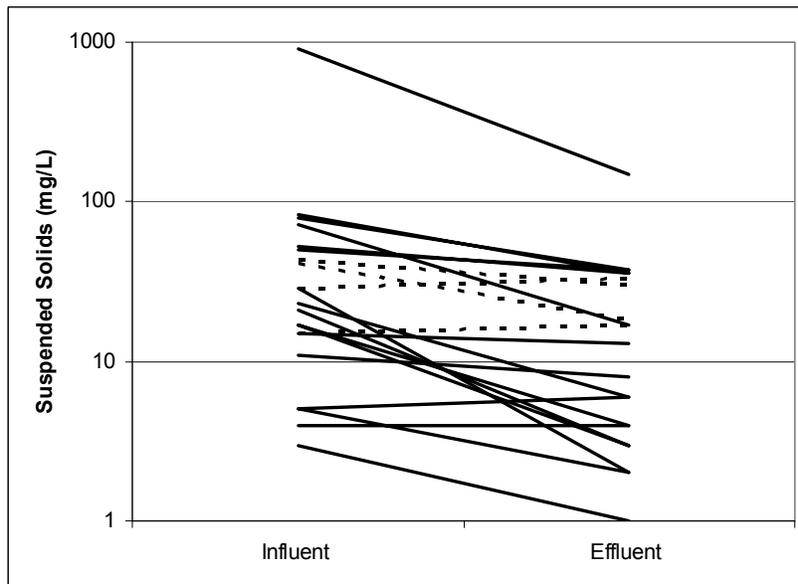
Figure 5-6: Paired influent and effluent suspended solids concentrations.
