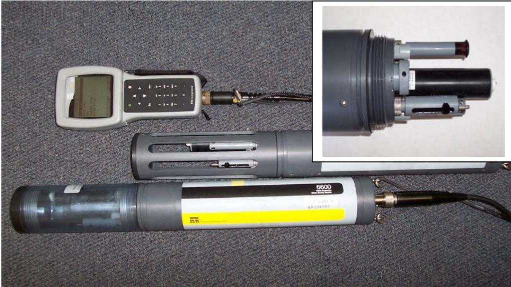
**Figure 4-16: YSI 6600 sondes and data logger, Inset – Close look at the sensors.**
