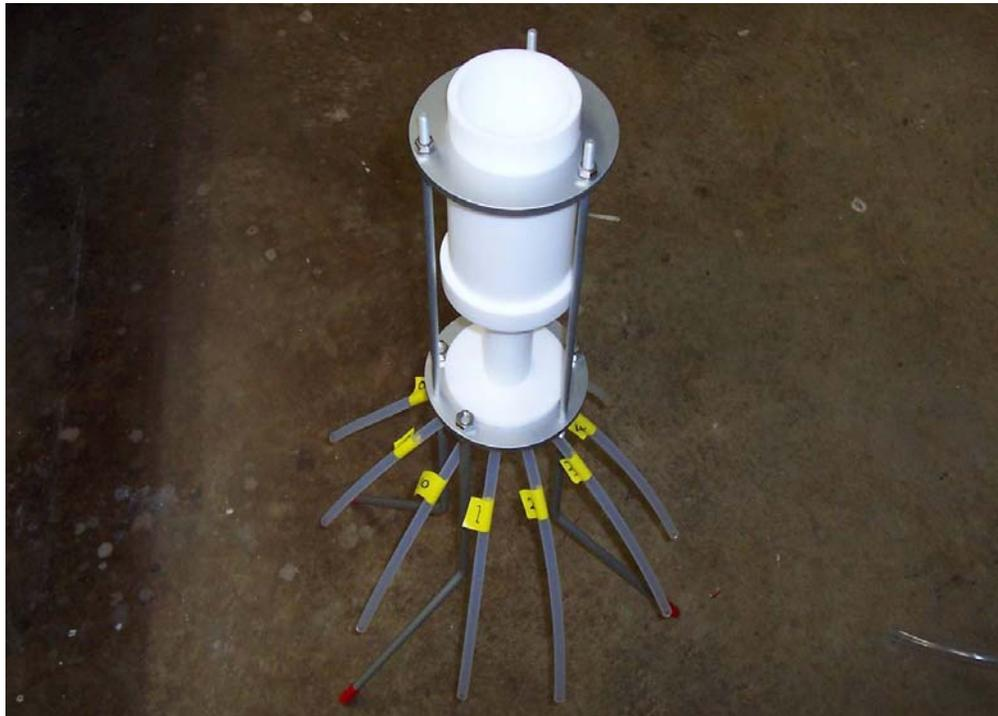
**Figure 4-11: Decaport cone splitter.**
