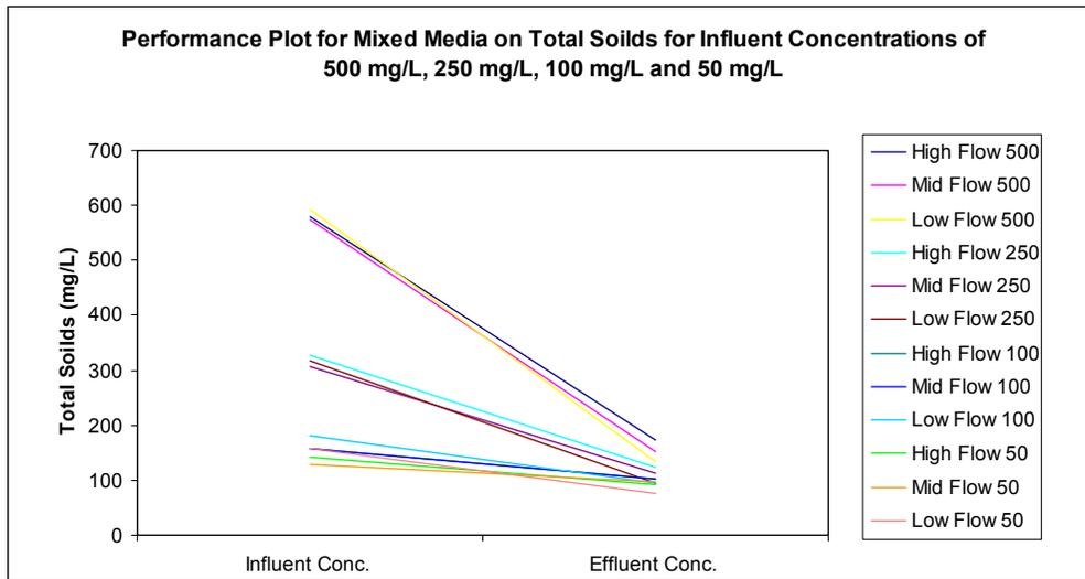
Figure 4-12: Performance plot for mixed media for total solids at influent concentrations of 500 mg/L, 250 mg/L, 100 mg/L and 50 mg/L.
