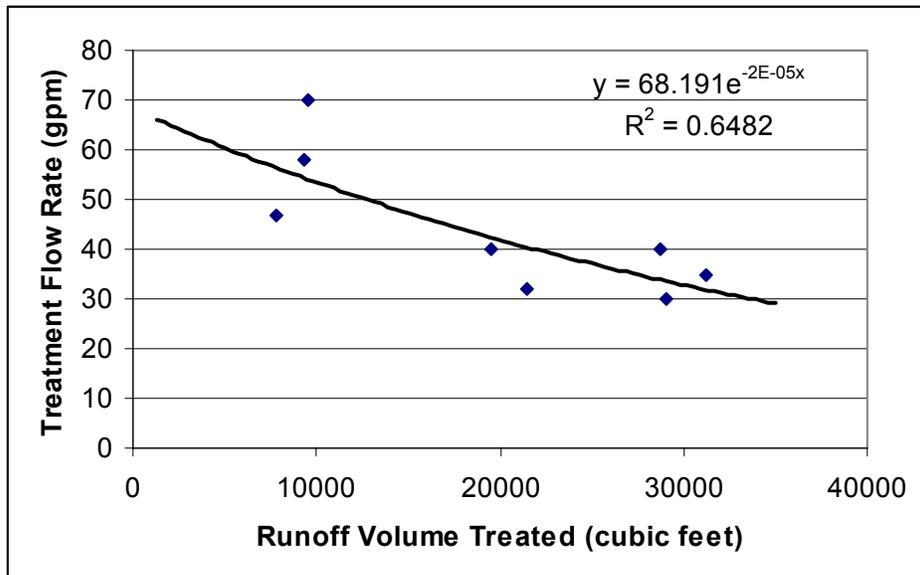
Figure 4-32: Up-Flo™ Filter treatment rate with runoff volume treated.
