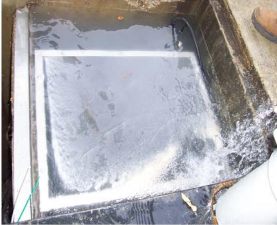
**Figure 4-9: Feed pollutant dispersing through filtration chamber**
