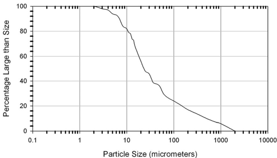
**Figure 3-11: Observed particulate matter size distribution in runoff water at Tuscaloosa test site.**
