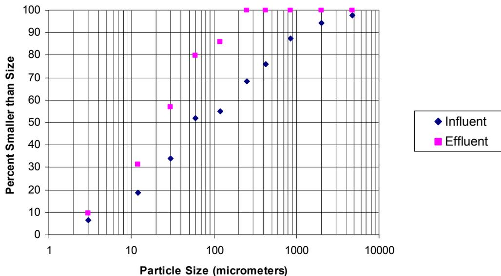
Figure 5-11: Particle size distributions for influent and effluent solids.
