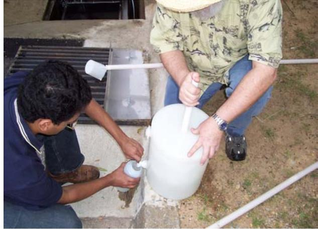
**Figure 4-10: Sample splitting using churn splitter**
