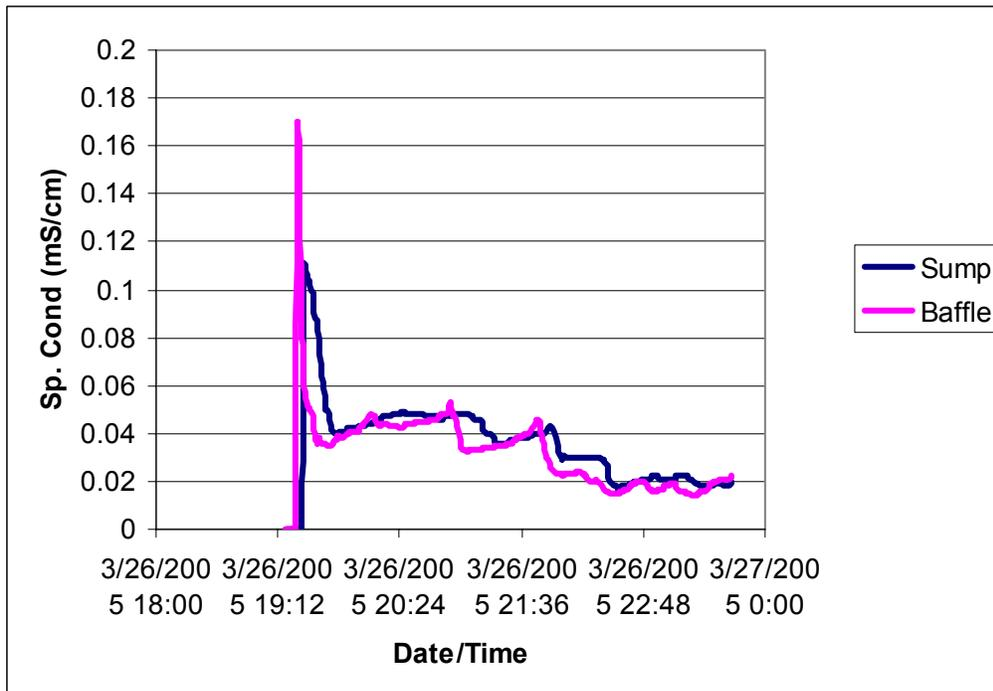
Figure D-2: Comparison of Specific Conductivity for Storm Event on March 26, 05
