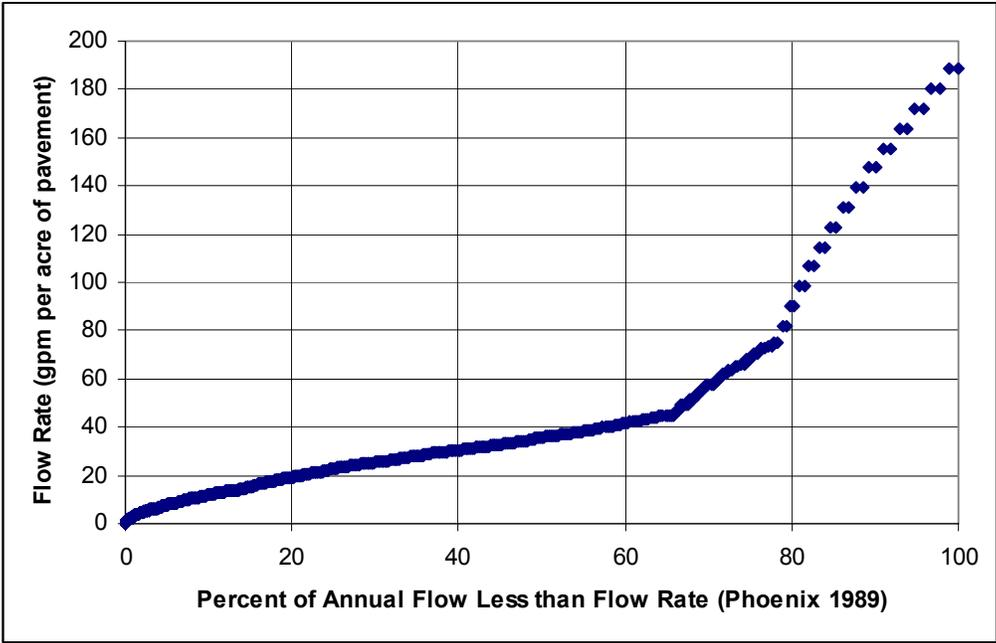
Figure 5-14: Treatment flow rates needed for Phoenix, AZ.
