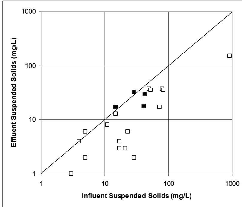
Figure 5-5: Scatterplot of observed influent and effluent suspended solids concentrations (filled symbols are events that had minor filter bypasses).
