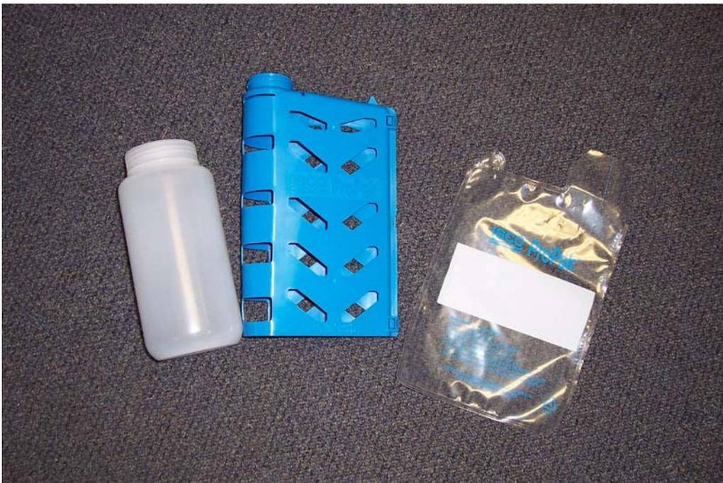
**Figure 4-17: ISCO Propack, Propack holder and Nalgene bottle used to store samples.**
