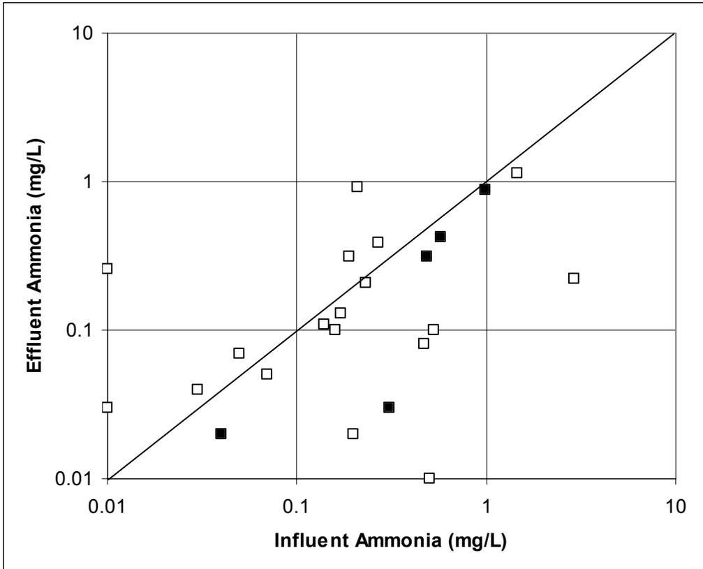
Scatterplot of observed influent and effluent ammonia concentrations (filled symbols are events that had minor filter bypasses).
