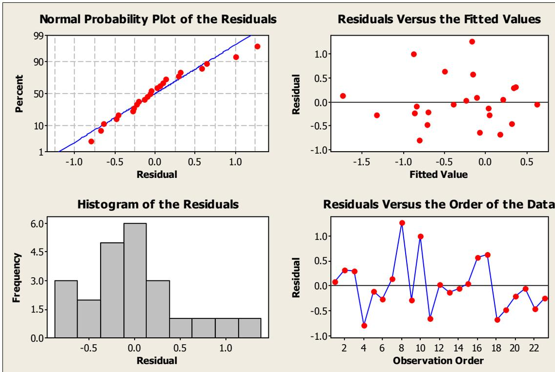
Residual analyses of fitted equation for 0.45 to 3  $\mu\text{m}$  particle size influent vs. effluent.
