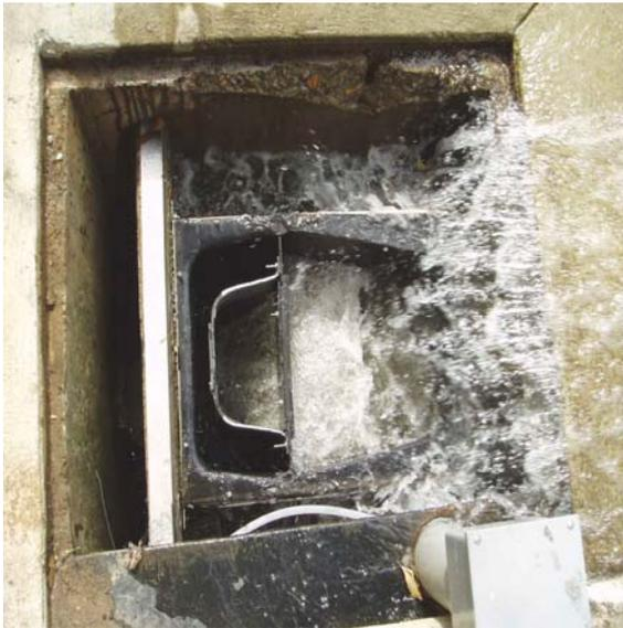
300 gpm into empty chamber with no overflow
