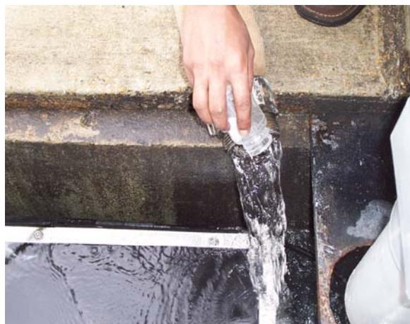
**Figure 4-8: Picture showing sediment addition**
