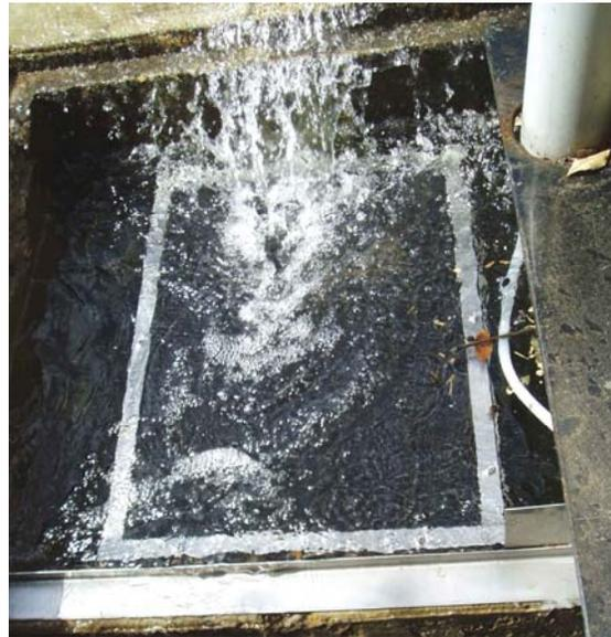
31 gpm flow with Mixed media at capacity
