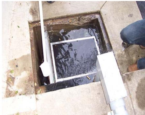
**Figure 4-6: Effluent sample collection**
