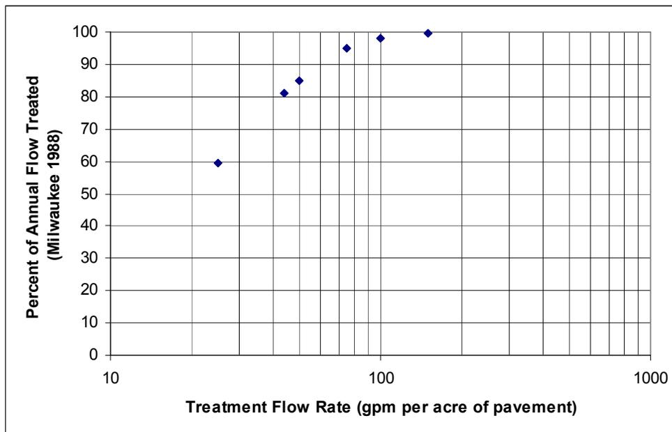
Figure 5-21: Treatment flow rates needed for Milwaukee, WI.
