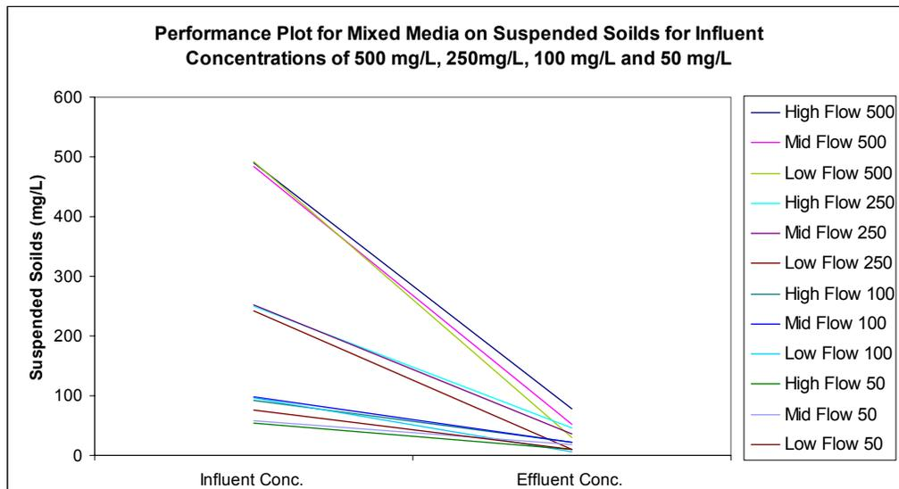
Figure 4-13. Performance plot for mixed media for suspended solids at influent concentrations of 500 mg/L, 250 mg/L, 100 mg/L and 50 mg/L.
