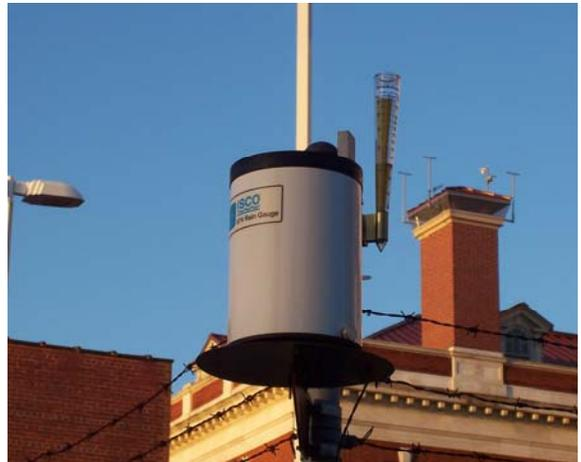
Figure 4-21: Tipping bucket and standard rain gauges installed at monitoring site.
