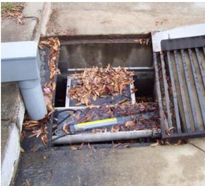
**Figure 4-24: Picture showing the influent sample tray and the sonde.**
