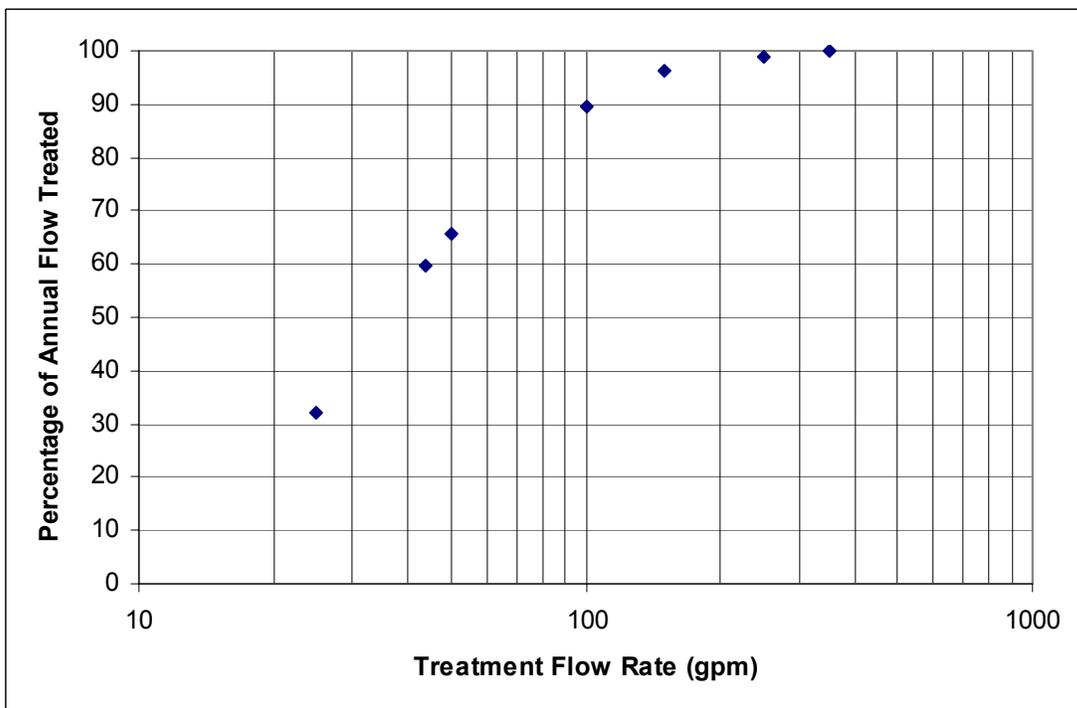
Figure 5-2: Treatment flow rate and percentage of annual flow treated for Tuscaloosa, AL, test site.
