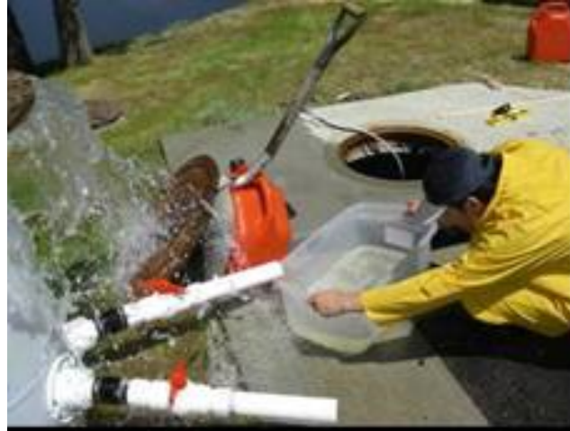
Figure 1.5 Pumped river water is discharged from splitter barrel to the 42 L (11 gal) plastic tray.
