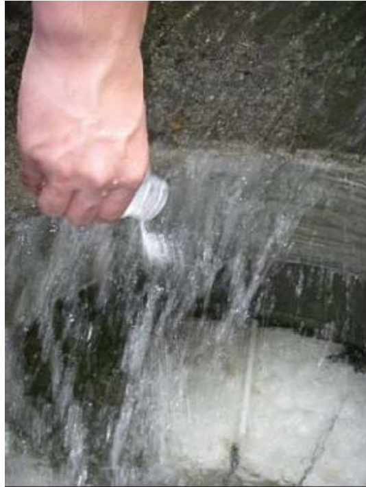
Figure 1.8 Sediment mixture was manually and consistently added to the Influent water over the 30 minutes test period.
