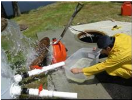
Figure 5. Pumped River water is discharged from splitter barrel to the 11 gallon plastic tray.
