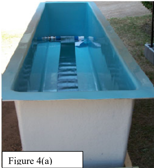
Figure 4. SmartDrain™ installations procedures in a fiberglass trough 3m long and 0.6 x 0.6m in cross section.
