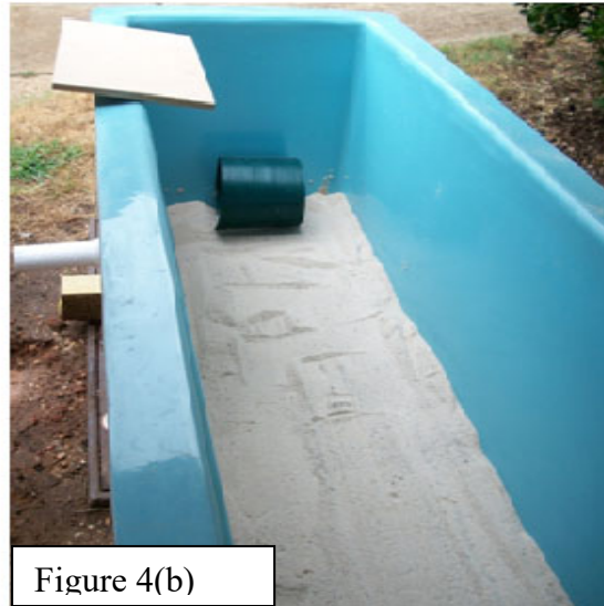
Figure 4. SmartDrain™ installations procedures in a fiberglass trough 3m long and 0.6 x 0.6m in cross section.
