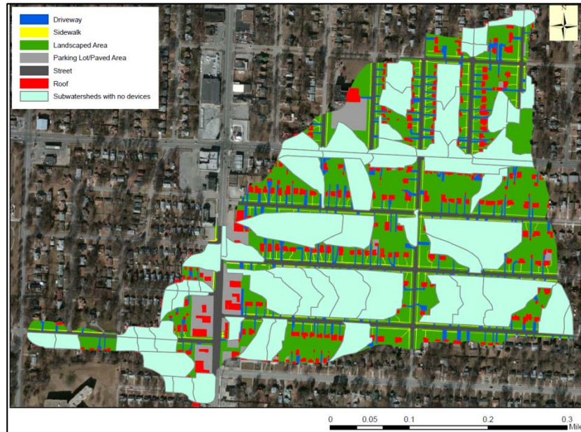
Figure X.4 Areas receiving surface stormwater control before being discharged into the combined sewer.
