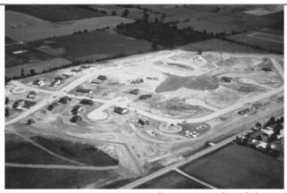
Most construction sites are characterized with large expanses of unprotected soil, even after utilities are installed (WI DNR photo)
