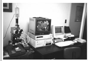
Research light microscope with automatic video analyses of particles
