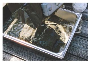
Figure 1-12. Typical Urban Stream Sediment (mostly silts and clays, little coarse material)
