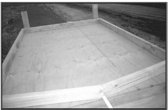
Figure 6-55. Auckland Regional Council rainfall-driven chemical dosing system, top plywood catchment tray (Beca Carter Hollings & Ferner Ltd, undated).
