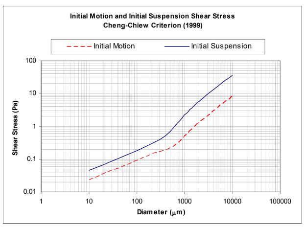
Figure 4-19. Initial motion and suspension of particles (specific gravity of 2.5) in flowing water as a function of shear stress (Avila 2008).
