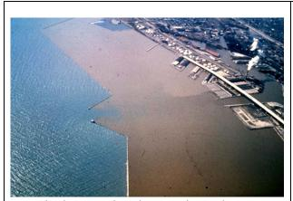
Outer harbor at Milwaukee in Lake Michigan frequently shows excessive turbidity from Kinnickinnic, Menomonee, and Milwaukee Rivers discharges during moderate to heavy rains. This has led to numerous investigations to identify the source of the sediment.
