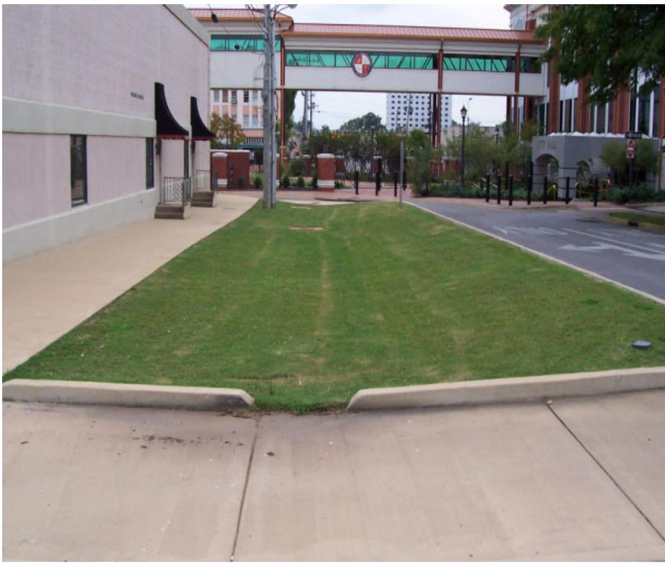
Fig. 62. Picture showing the outdoor test swale (116 ft (35.3 m) in length draining 0.1 acres (390 m<sup>2</sup>) of paved road)
