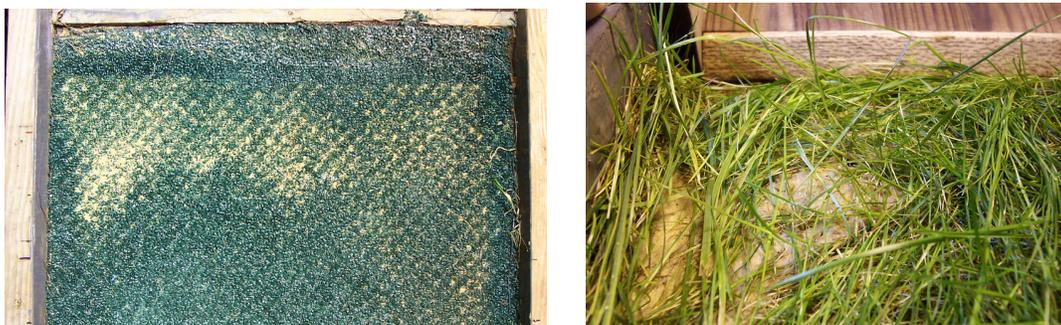
Fig. 32. (*left*) Picture showing sand accumulation on the synthetic turf swale
