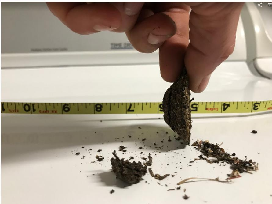
Figure 2.6 Compromising debris removed from funnel after a large rain
