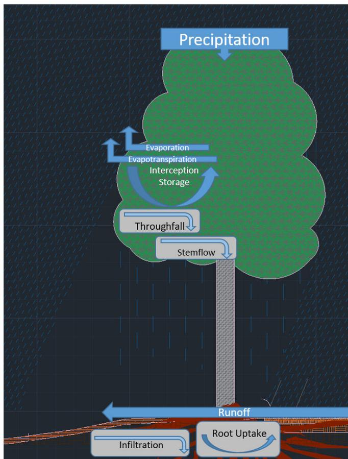
Figure 1.4-Illustration of hydrologic process for rainfall partitioning
