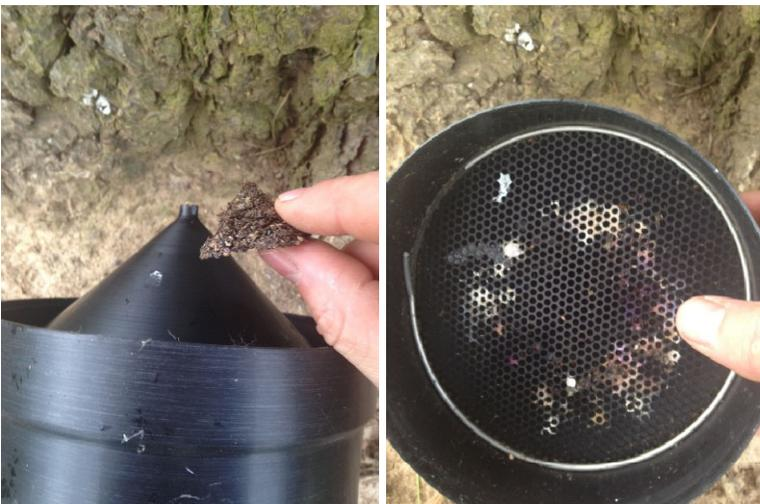
Figure 2.5- Clogging impacts water flow through the tipping bucket. Over time ponding will form in the funnel as the debris builds (left). Birds droppings commonly clog the screens leaving passed seeds in the funnel. (right)
