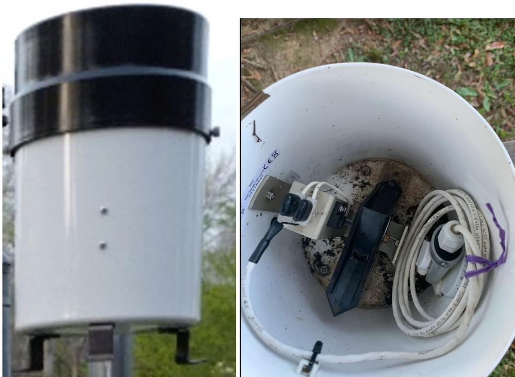
Figure 2.4- HOBO Data Logging Rain Gauge RG3
