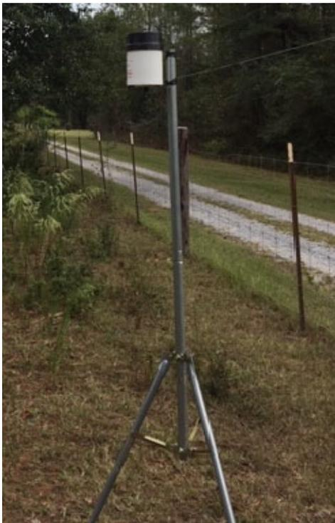
Figure 2.3- HOBO data logging rain gauge RG3
