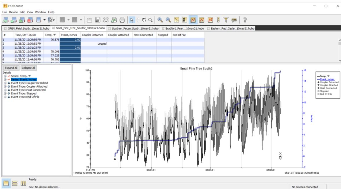
Figure 2.7 – HOBOWare® software display for cumulative rainfall (in) and temperature (°F) data for six months under a pine tree
