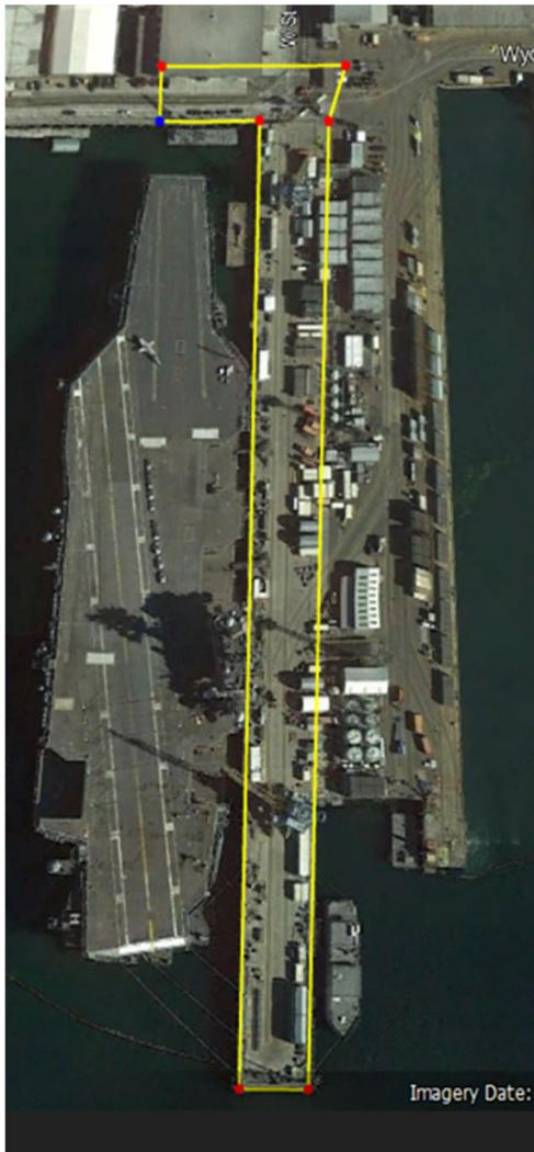
Aerial drainage map of Pier B site in PSNS with drainage represented by yellow lines
