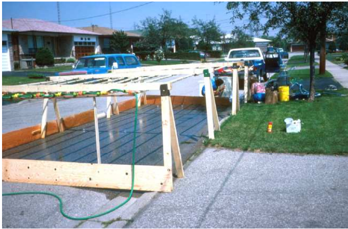
Figure 12.8 Small-scale washoff test setup in Toronto (Pitt 1987).
