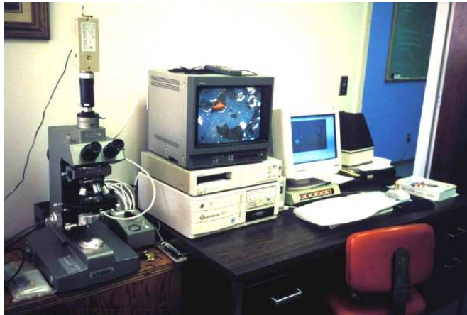
Figure 12.10 Light microscope and video capture that can be used to measure particle sizes from washoff experiments.
