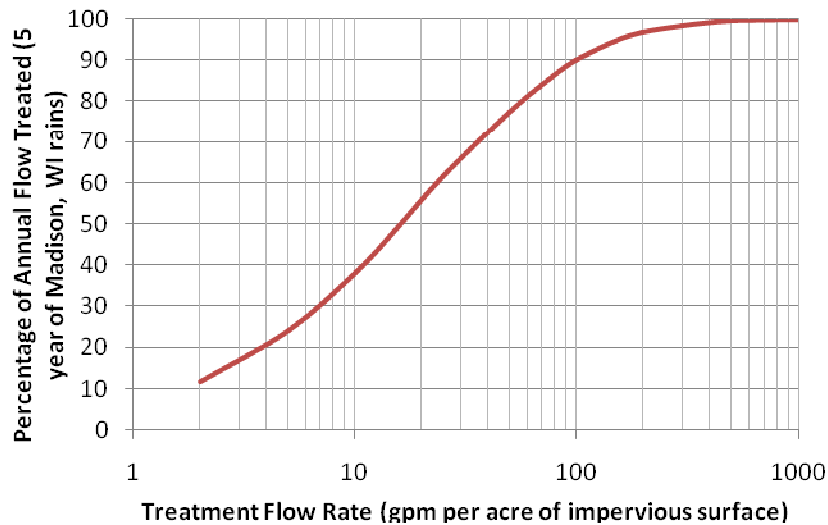
Figure X.2 Percentage of annual flows treated for different treatment flow rates (no storage).
