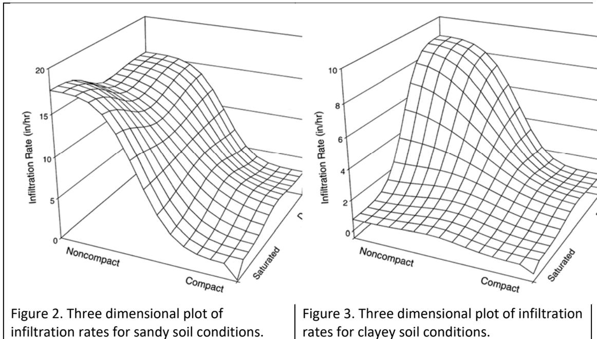
Figure 2. Three dimensional plot of infiltration rates for sandy soil conditions.
