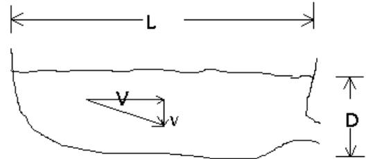
The water velocity is equal to the water volume discharge rate (Q, such as measured by cubic feet per second) divided by the pond cross-sectional area (a = depth times width: DW, in equation (2):
