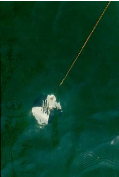
Secchi Disk used to Measure Water Turbidity
