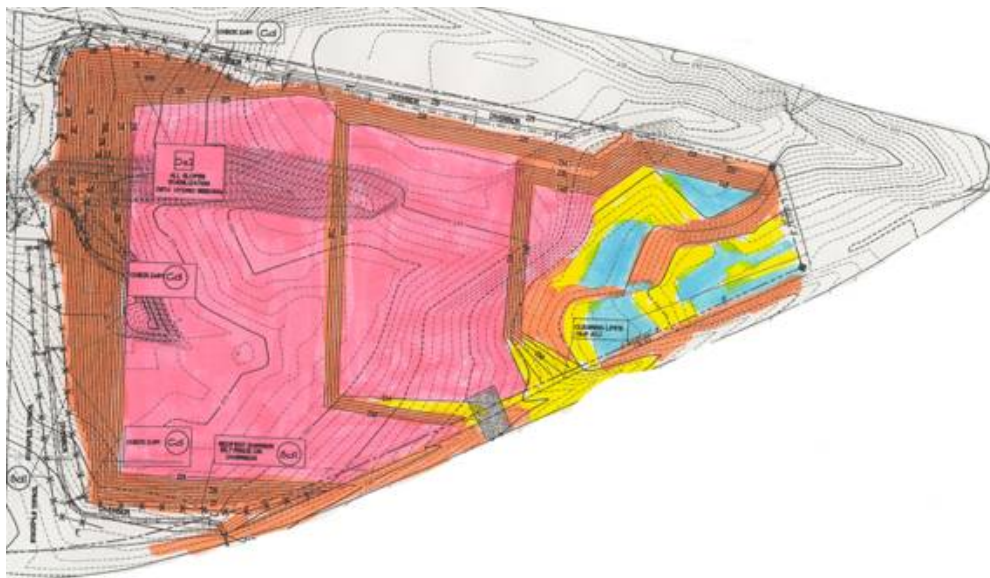
Figure 2-2. Evaluation of final grading plan topography (solid contour lines) for erosion hazards (orange: >10% slopes and high hazard; yellow: 5 to 10% slopes and high hazard; blue: 2 to 5% slopes and moderate hazard; pink: <2% slopes and low hazard).
