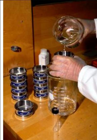
Cascading sieves (with total solids analyses after each sieve)
