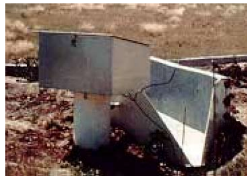
H-flume (with Instrument Shelter)
