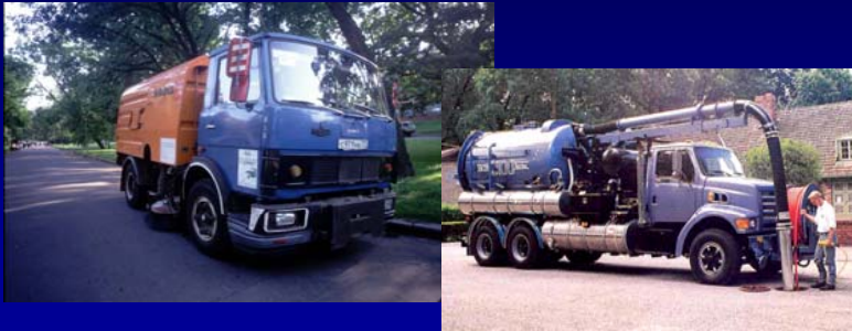
Street and catchbasin cleaning, and inlet controls most effective for smaller rains in heavily paved areas.
