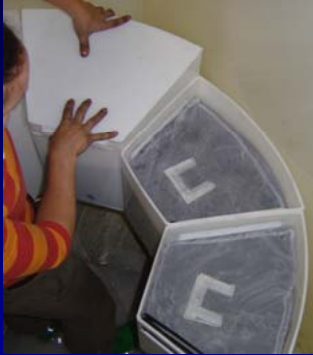
Assembling Upflow Filter modules for lab tests
