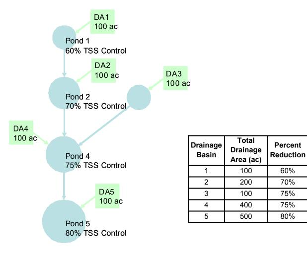
Scenario A – Downstream-most pond has highest TSS reduction efficiency
