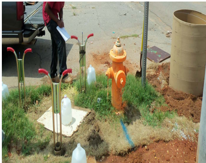
Figure 3. Double Ring Infiltration Measurement Installations at Test Site 3.
