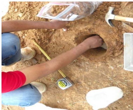
Figure 2. Photographs showing the infiltration measurement setup and in-situ soil density measurement at Shelby park biofilter.
