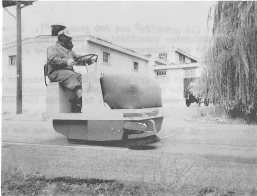
Fig. 2.3 Vacuumized Sweeping (Tennant Model 80) on Asphaltic Concrete.
