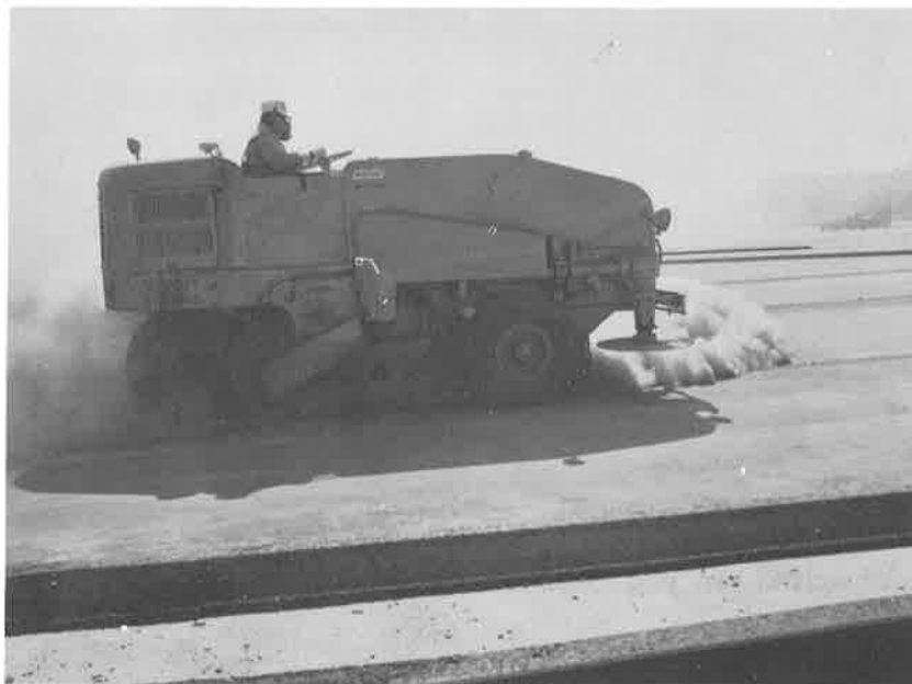
Fig. 2.1 Motorized Sweeping (Wayne Model 450) on Portland Cement Concrete.
