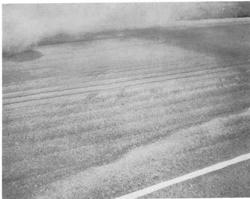
Fig. 4.6 Ridges of dry synthetic fallout material left on surface after one pass of the air broom. Initial mass of 147 \text{ gms/ft}^2 .
