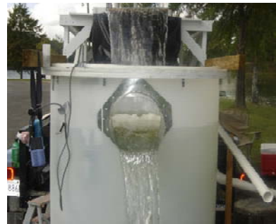
Figure X.2. Placement of sediment at 25 cm below the outlet (left). Performing scour test (right).
