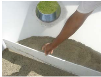
Figure X.2. Placement of sediment at 25 cm below the outlet (left). Performing scour test (right).
