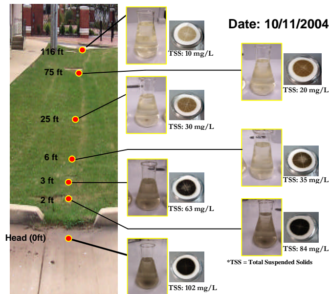
Figure 11.5 Sampling locations at the outdoor swale monitoring site (Example sediment samples from 10/11/2004)
