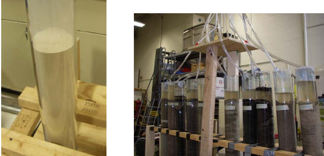
Figure 3-10. Long-Term Column Breakthrough Testing Setup. Left: Glass column under construction. Right: Complete column testing setup.
