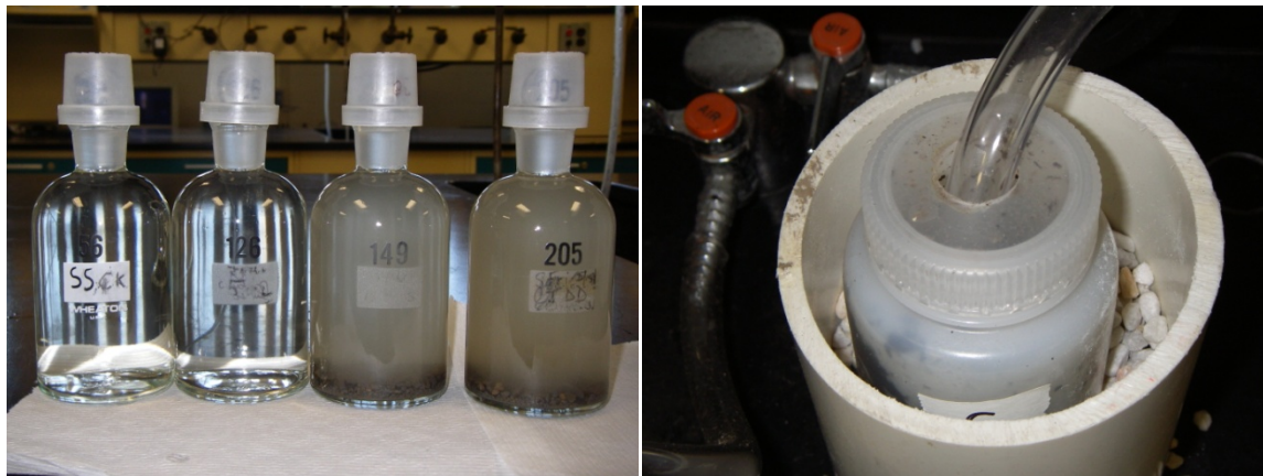
Figure 3-14. Anaerobic Bottles (left) and Aerobic Bottles (right) during Exposure
