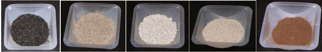
Figure 1. Media (from left to right): GAC, Rhyolite Sand, Site Zeolite, Surface Modified Zeolite, Sphagnum Peat Moss
