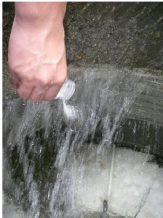
Figure 8. Sediment mixture was manually and consistently added to the influent water over the 30 minute test period.
