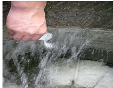
**Figure 8. Sediment mixture was manually and consistently added to the influent water over the 30 minute test period.**
