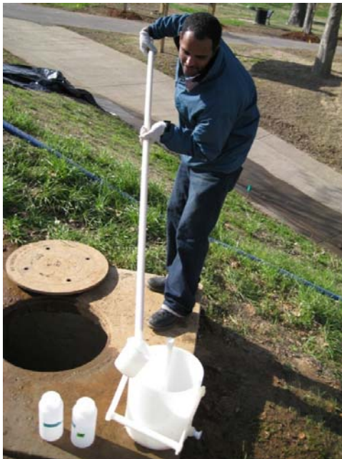
Samples are taken from the effluent box after the Up-Flo® Filter
