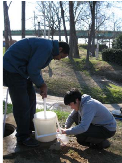
Sample splitting using churn splitter
