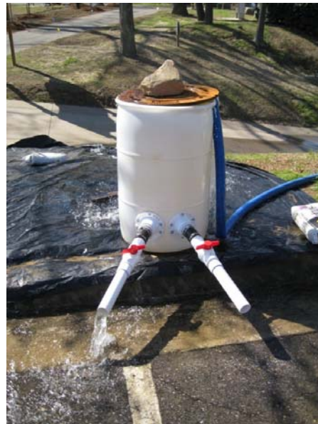
River water is pumped into the plastic flow splitter barrel (low flow test)
