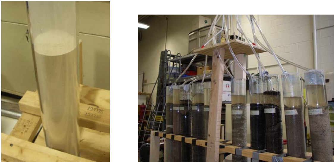
Figure 2. Long-Term Column Breakthrough Testing Setup. Left: Glass column under construction. Right: Complete column testing setup.
