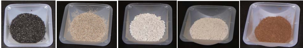
Figure 1. Media (from left to right): GAC, Rhyolite Sand, Site Zeolite, Surface Modified Zeolite, Sphagnum Peat Moss
