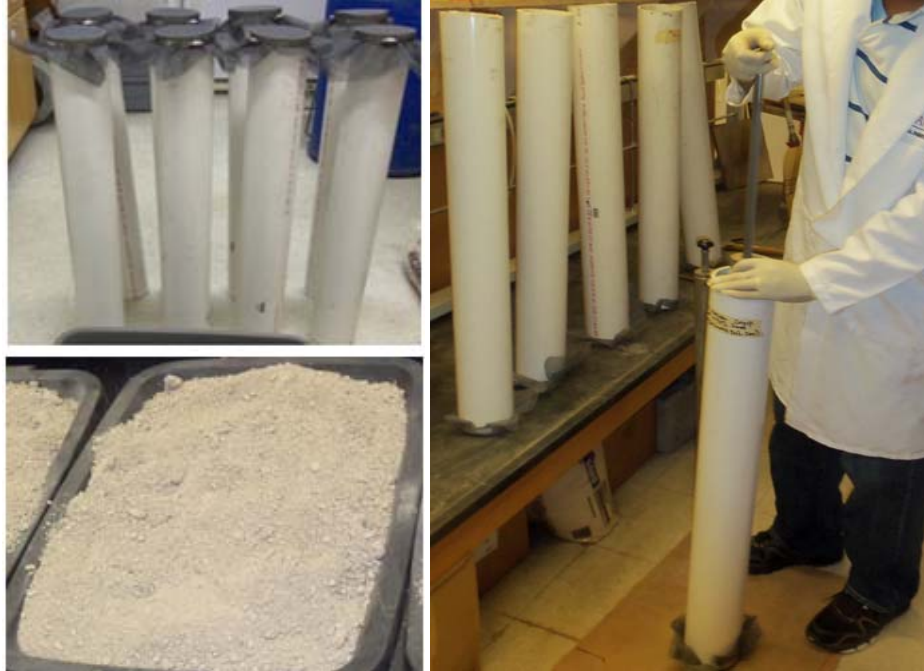
Figure 112. Lab Column Infiltration Tests (Left To Right): Bottom of the Columns Secured with a Fiberglass Window Screen (Upper Left), Biofilter Media (Lower Left), and Media Compaction.
