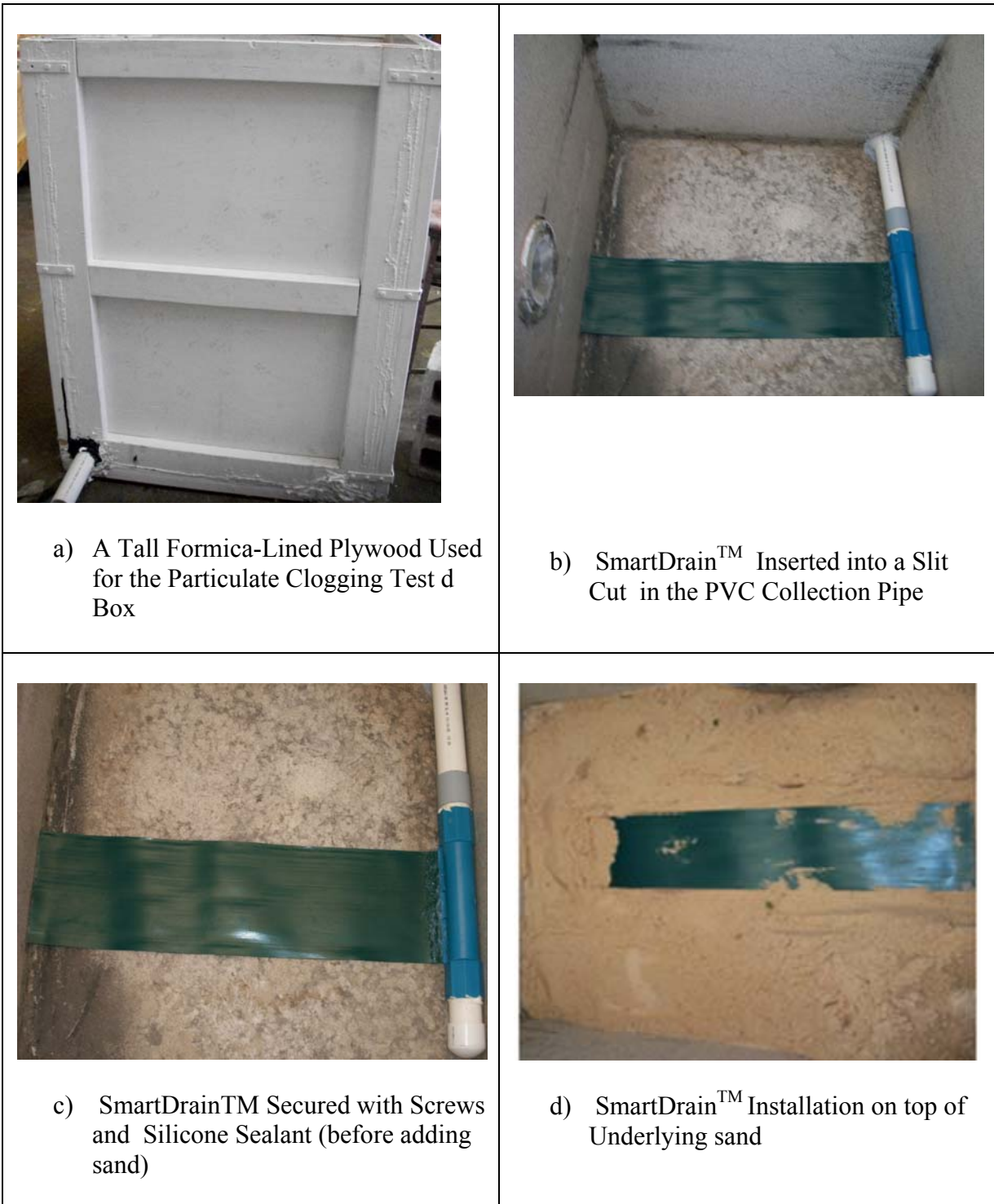
Figure 25. SmartDrain™ Clogging Test Setups with the Deep Water Pilot-Scale Biofilter.
