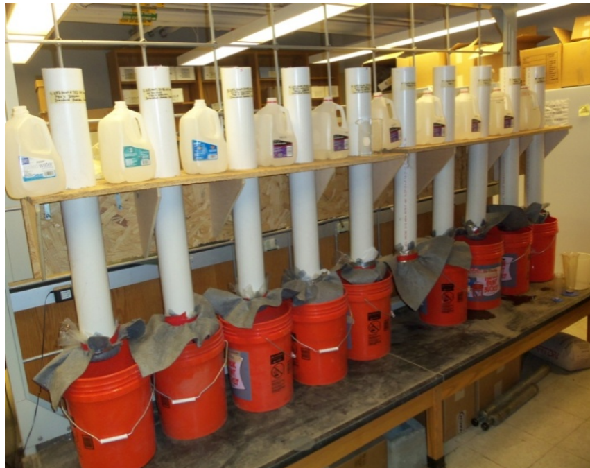
Figure 113. Laboratory Column Setup for Infiltration Measurements.
