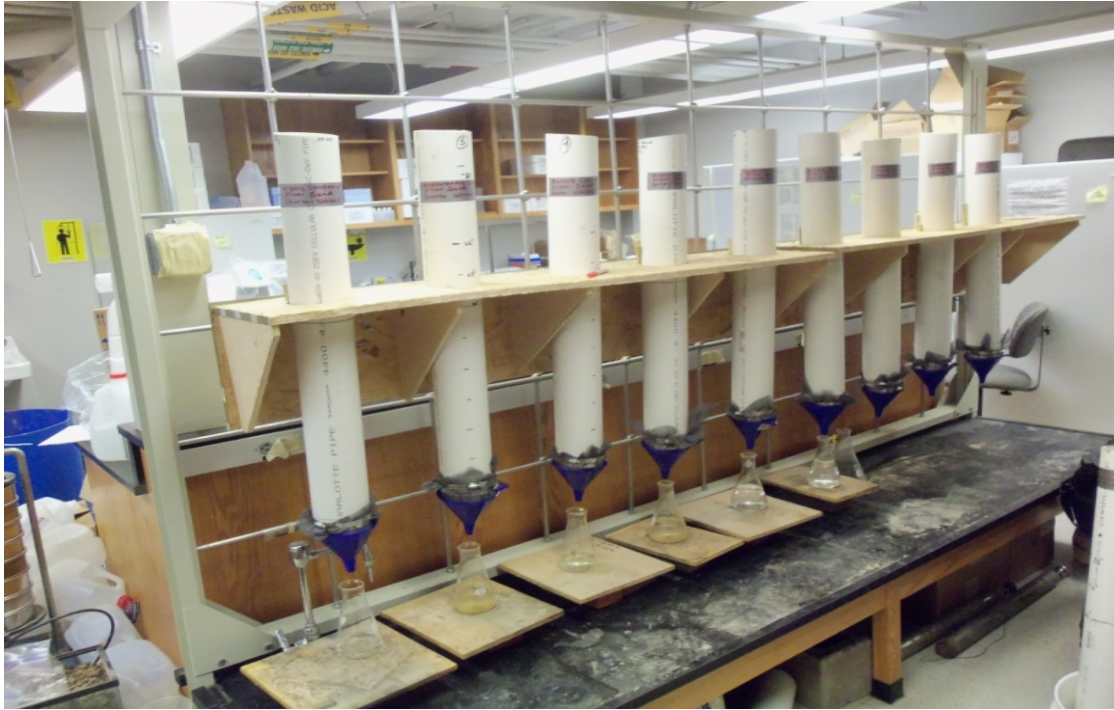
Figure 67. Laboratory Column Setup.
