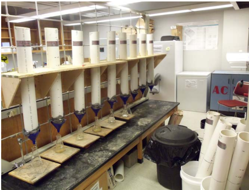
Figure 94. Laboratory Setup for Nine Soil Infiltration Test Columns.
