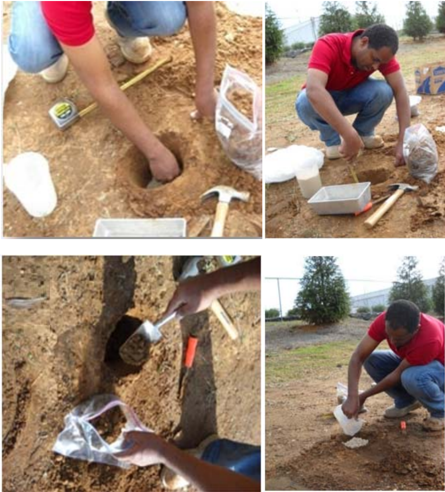
Figure 62. Photographs Showing the Infiltration Measurement Setup and In-Situ Soil Density Measurements at Shelby Park Biofilter.
