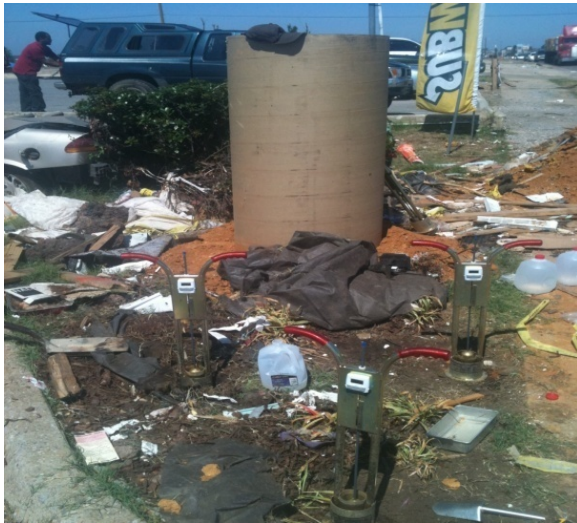
Figure 92. Borehole Marking, Borehole Drilling, Double-ring and Borehole Infiltration Measurement Installations at McDonalds on 15 th St. and 6 th Ave. Ave. E., Tuscaloosa, AL.
