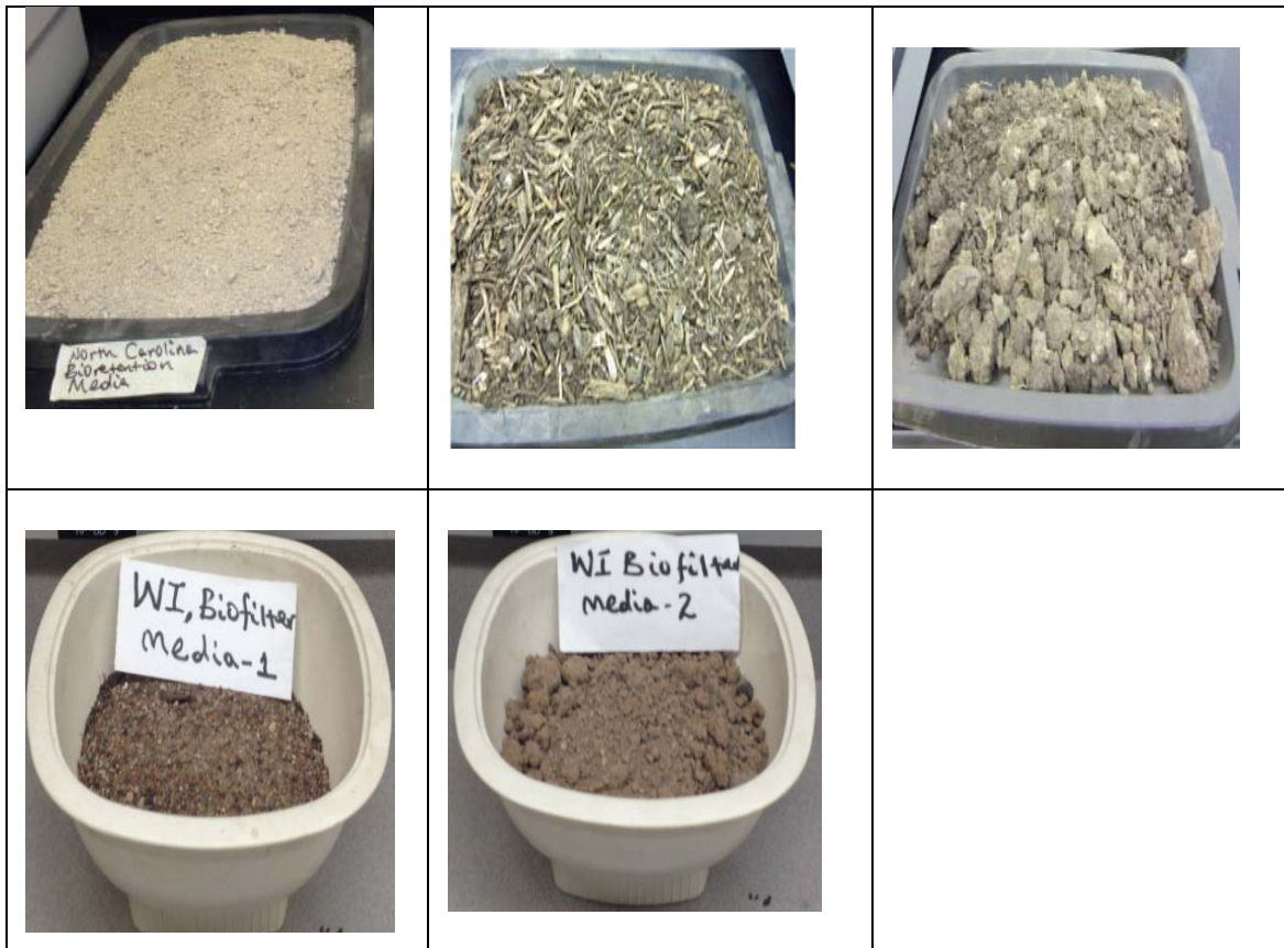
Figure 110. Biofilter Media Mixtures (From Left To Right): North Carolina Biofilter Media, Kansas City Biofilter Media from Test Sites 1 and 2, and Wisconsin Biofilter Media from Test Sites 1 and 2.
