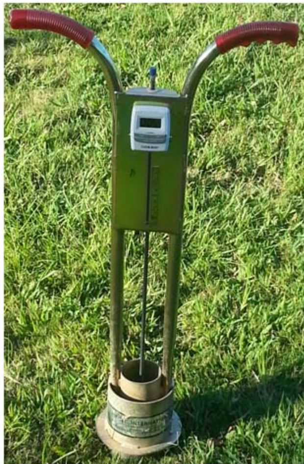
Figure 63. A Close Up of Turf-Tec Infiltrometer (available from Turf-Tec International)
