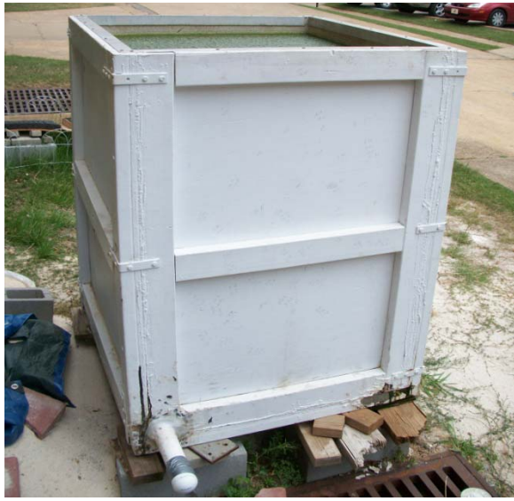
a) A Tall Formica-Lined Plywood Box Used for the Biofouling Test
