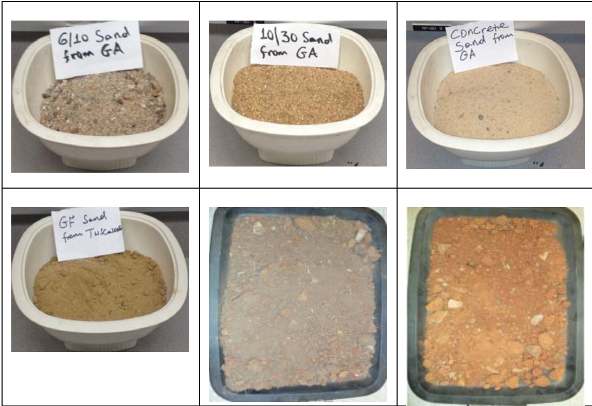
Figure 108. Sand Media Obtained from Atlanta Sand and Supply (From Upper Left to Upper Right), Sand from Ground Floor Sand Supplier, Northport, AL (Lower Left), Tuscaloosa Surface Soil and Tuscaloosa Subsurface Soils (Lower Middle and Lower Right).
