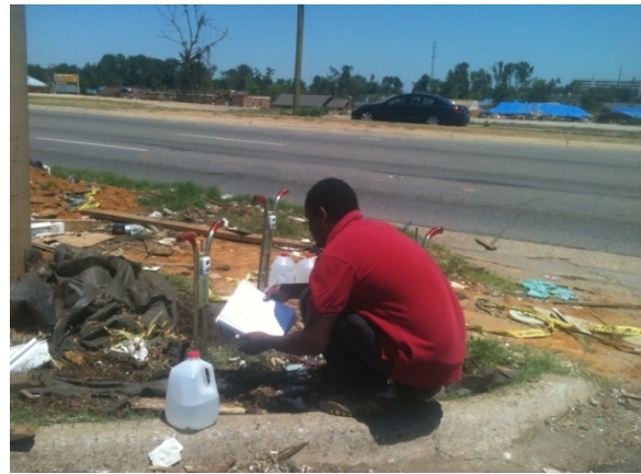
Figure 92. Borehole Marking, Borehole Drilling, Double-ring and Borehole Infiltration Measurement Installations at McDonalds on 15 th St. and 6 th Ave. Ave. E., Tuscaloosa, AL.
