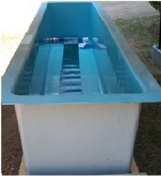
(a) SmartDrain™ Inserted into a Slit Cut in the PVC Collection Pipe and Secured with Screws and Silicone Sealant (before sand)
