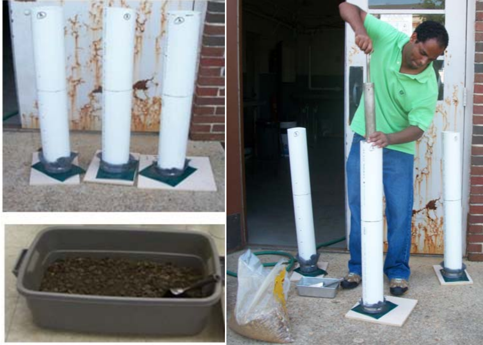
Figure 66. Lab Column Construction for Infiltration Tests (Left to Right): Bottom of the Columns Secured With a Fiberglass Window Screen (Upper Left), Soil Media (Lower Left), and Media Compaction.
