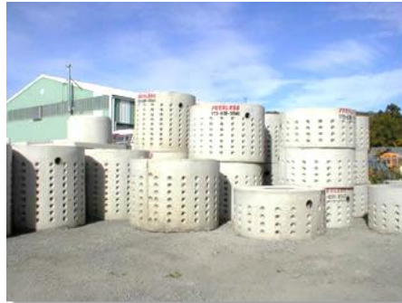
Figure 1.1 Peerless Concrete Products, Butler, NJ, supplies the dry wells to many of the sites in Millburn (photo from http://www.peerlessconcrete.com/ )
