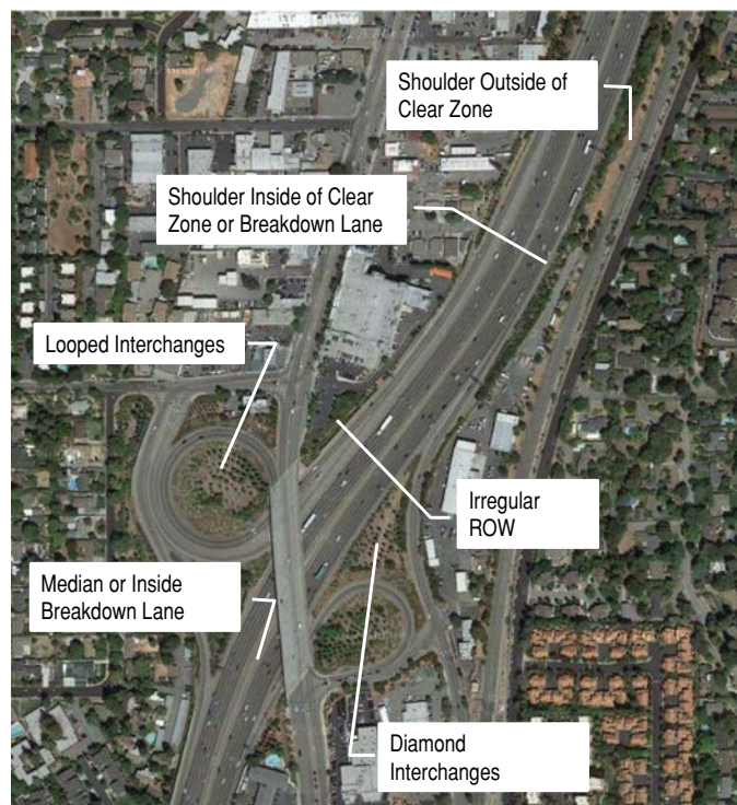
Figure 7. Key to common geometric opportunities within urban highway environment (hypothetical opportunities shown).
