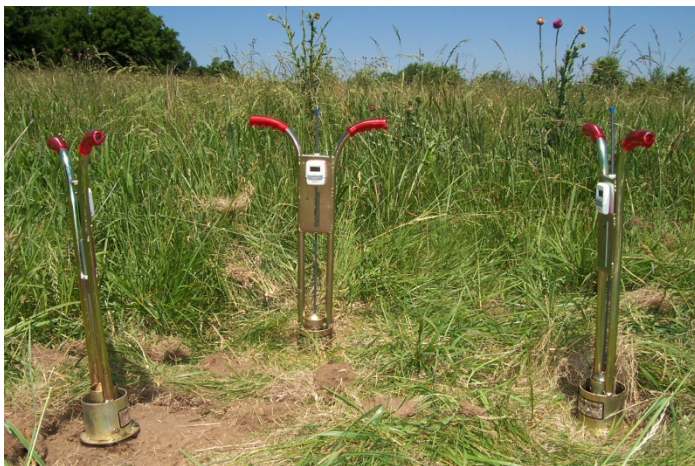
Figure 13. Three Turf-Tec infiltrometers for infiltration measurements in pre-development soils.
