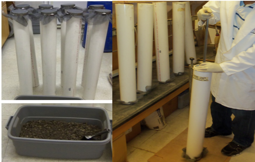
Figure 47. Lab column construction for flow test using Kansas City soil media: bottom of the columns secured with a fiberglass window screen, mixed soil media, and soil compaction.
