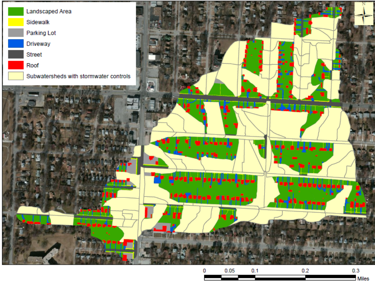
Figure 68. Map of test (pilot) area showing surface characteristics of areas not receiving stormwater treatment.
