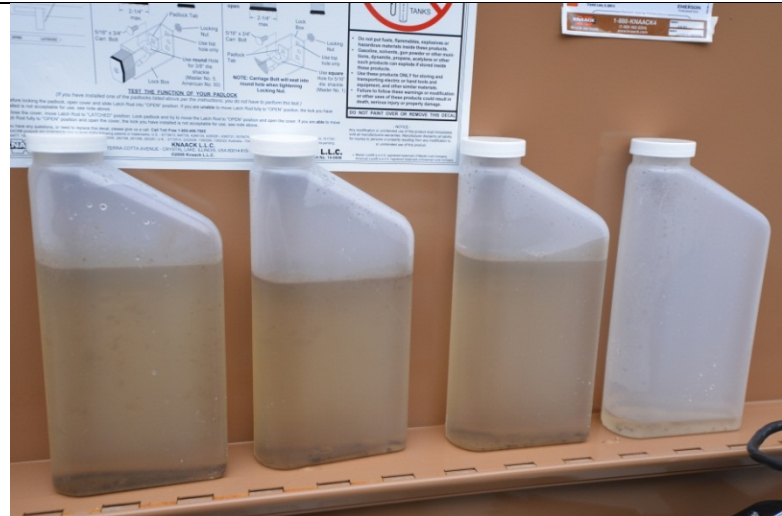
4 inlet samples from small rain of morning of Oct 25, 2012 (initial sample contains more sediment)
