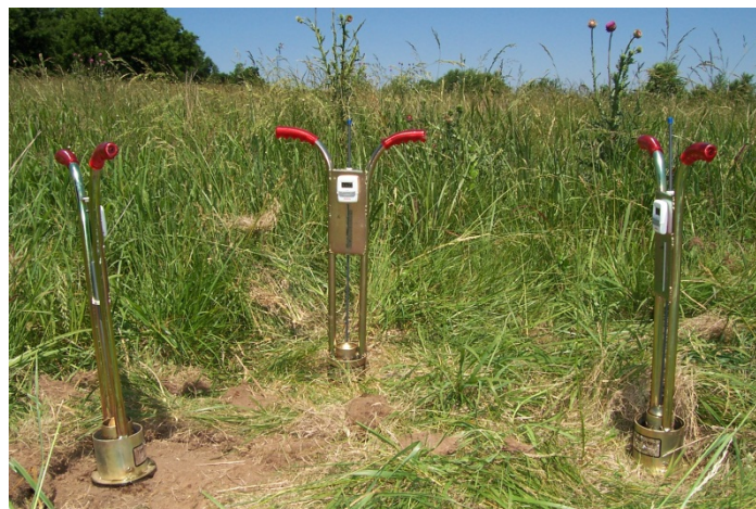
Figure 27. Set of three Turf-Tec infiltrometers for infiltration measurements in pre-development soils.
