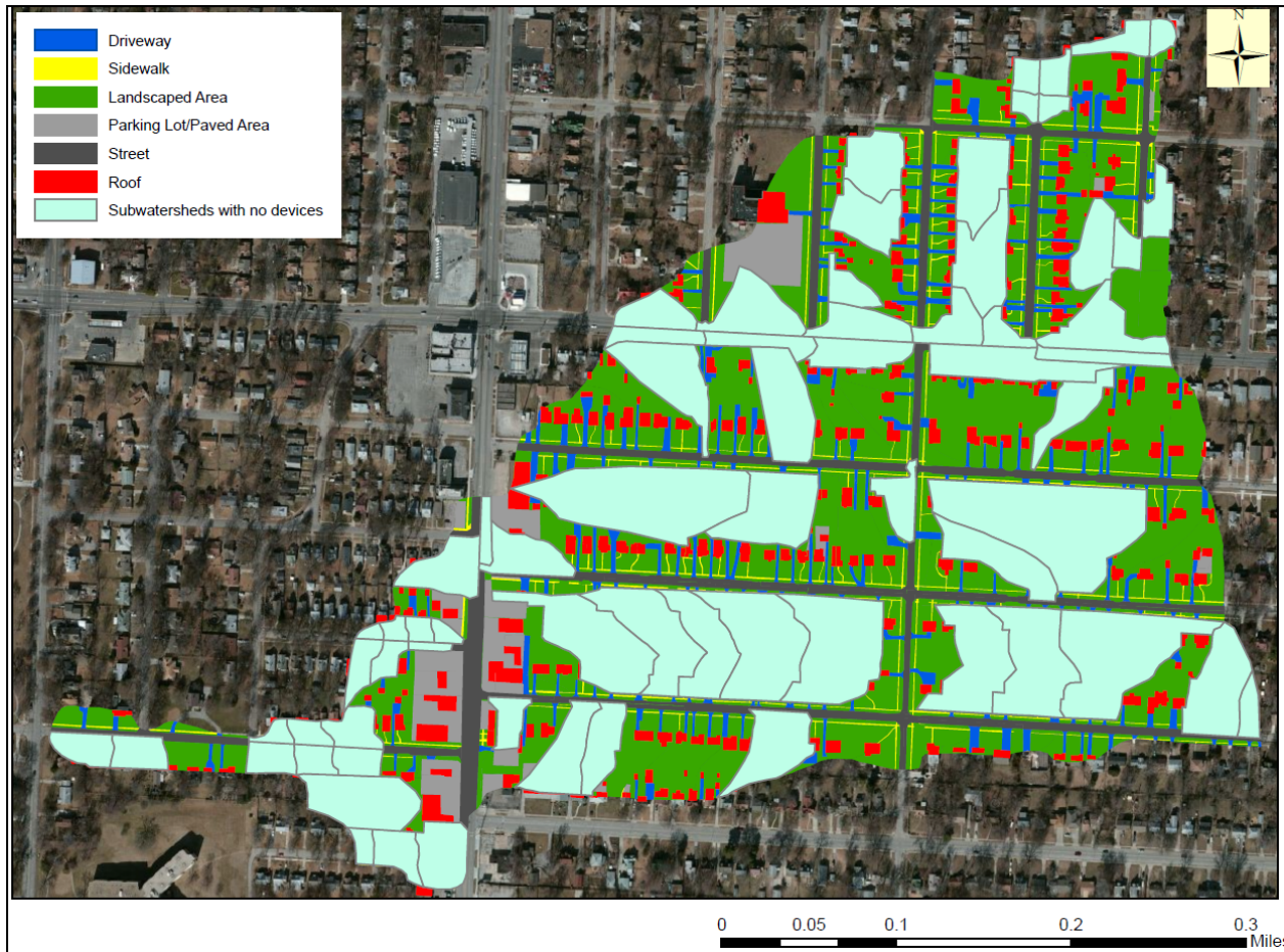
Figure 10. Areas receiving surface stormwater control before being discharged into the combined sewer.
