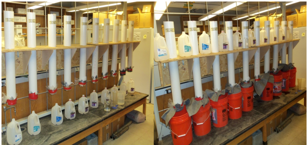
Figure 49. Laboratory column setup for porosity and infiltration measurements
