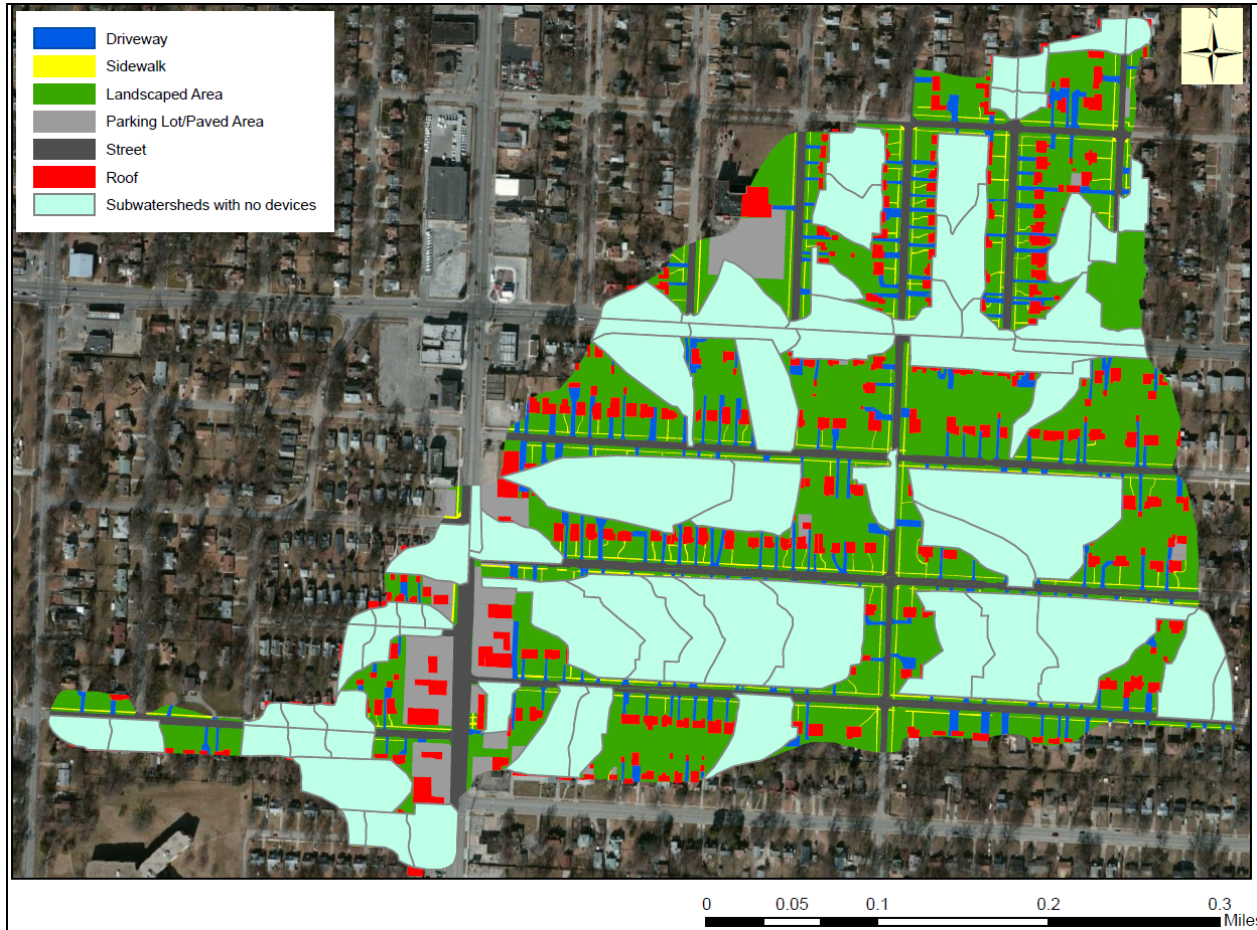
Figure 67. Map of test (pilot) area showing surface characteristics of areas receiving stormwater treatment.
