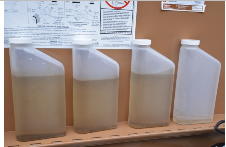
4 inlet samples from small rain of morning of Oct 25, 2012 (initial sample contains more sediment)
