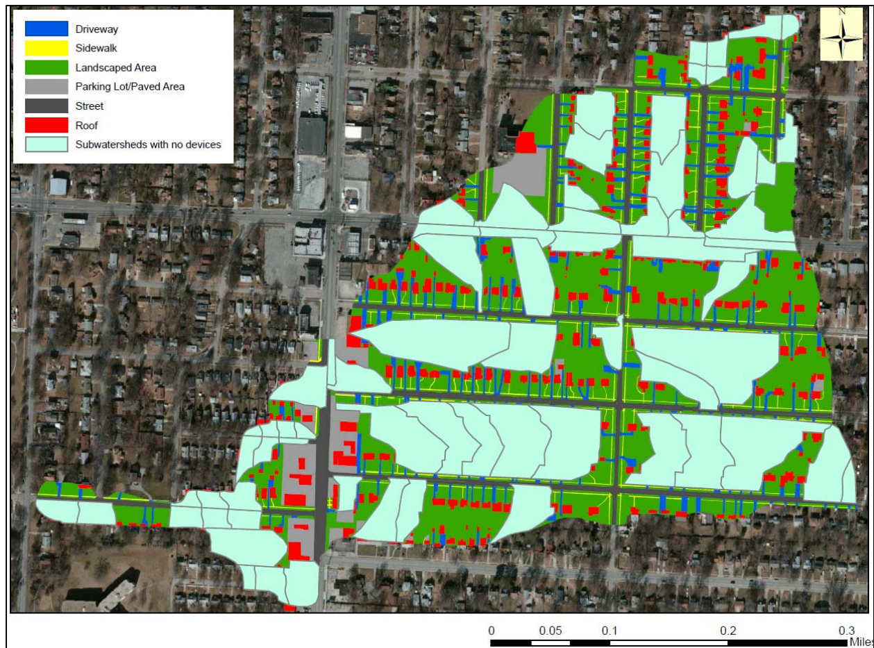
Figure 9. Areas receiving surface stormwater control before being discharged into the combined sewer.
