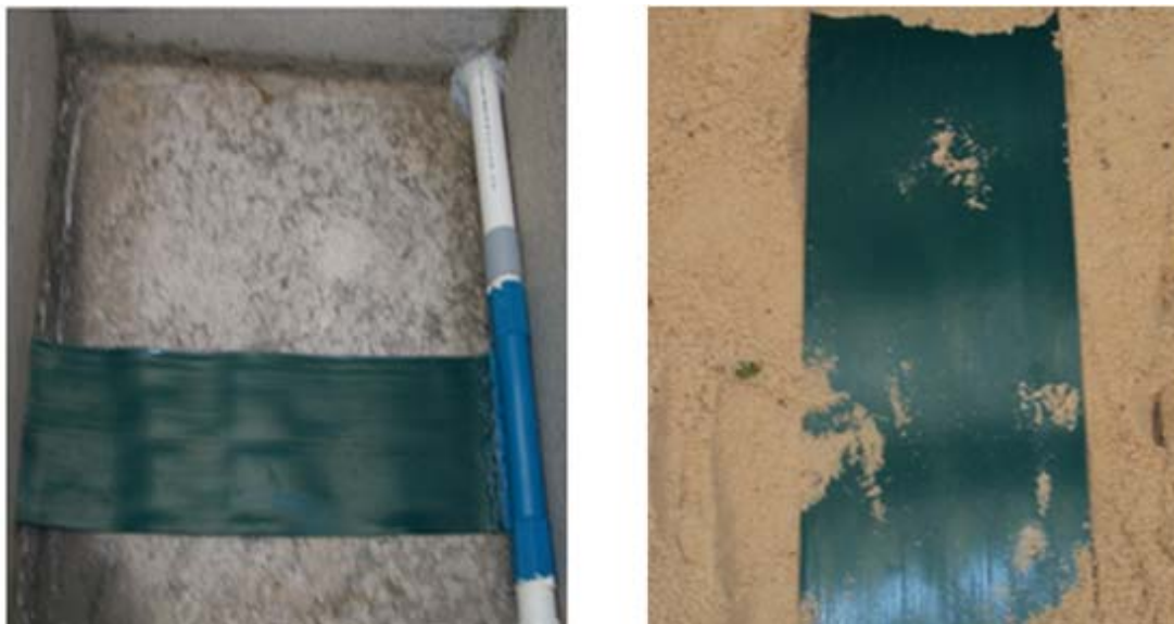
Figure 109. SmartDrain™ installation for the clogging test in the tall box.
