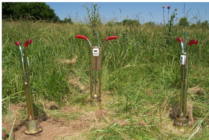
Figure 26. Set of three Turf-Tec infiltrometers for infiltration measurements in pre-development soils.
