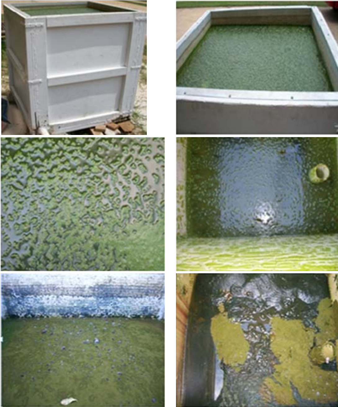
Figure 110. Algae in the test tank during the biofouling tests.
