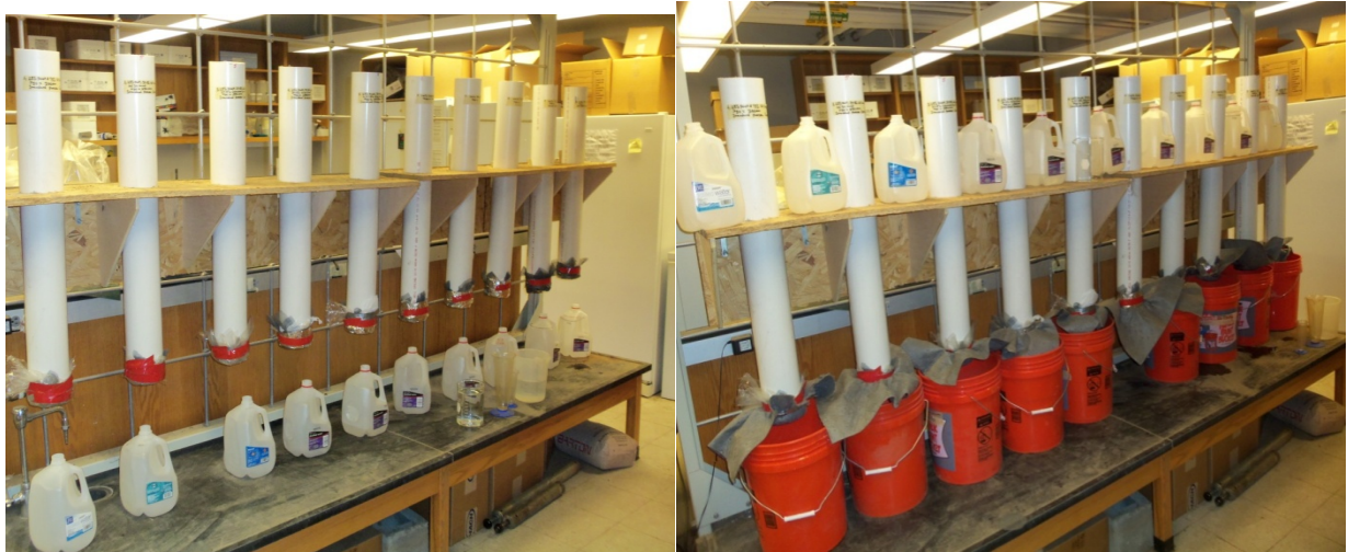
Figure 65. Laboratory column setup for porosity and infiltration measurements
