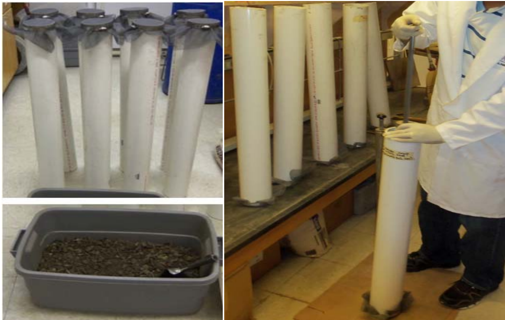
Figure 63. Lab column construction for flow test using Kansas City soil media: bottom of the columns secured with a fiberglass window screen, mixed soil media, and soil compaction.
