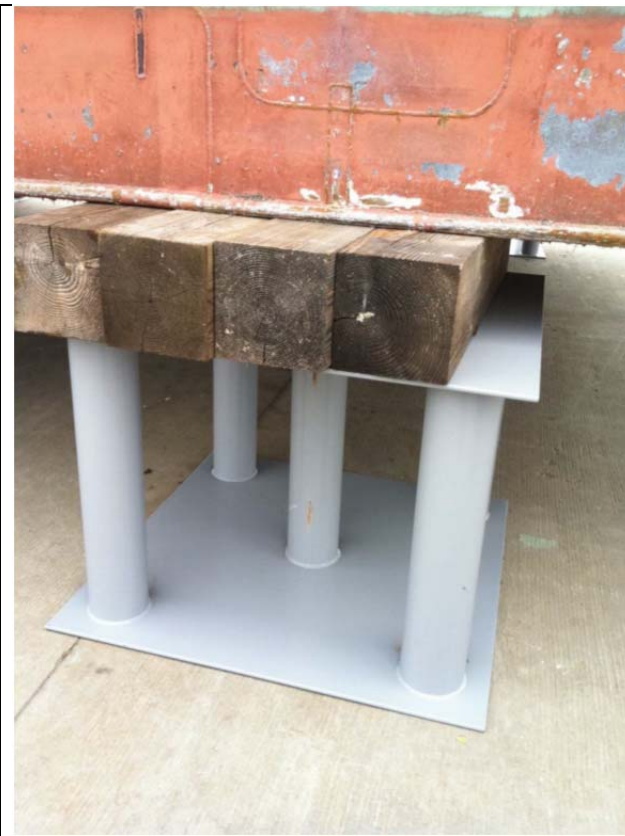
Photo 8: Painted metal barge support stands
