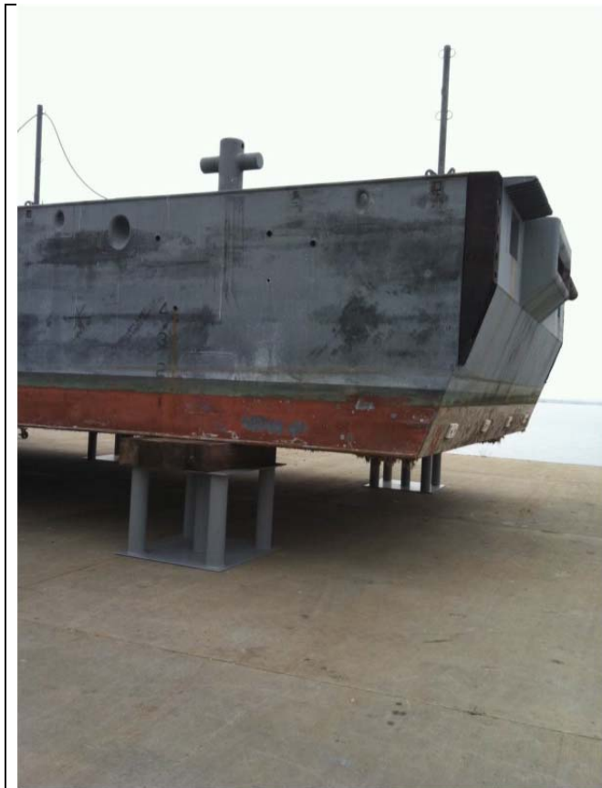
Photo 7: Barge supported by stands
