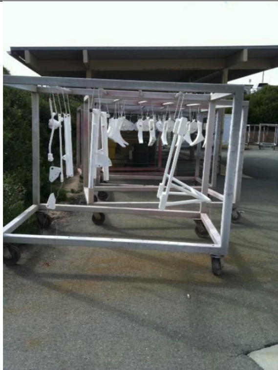
Photo 10: Galvanized drying rack for painted materials. Near Building 814 Industrial West
