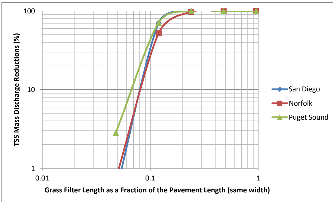
TSS mass discharge reductions for different lengths of grass filter strips.
