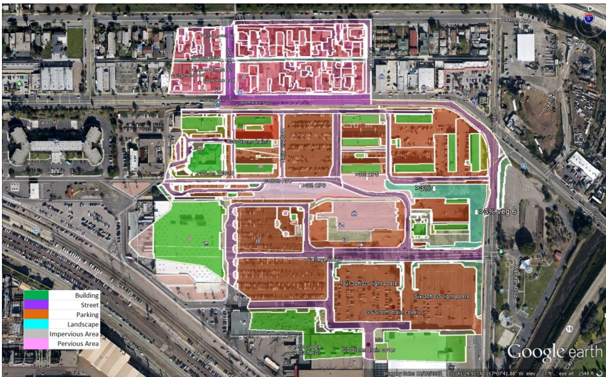
Drainage overview and Land use characterization for NBSD Outfall 72
