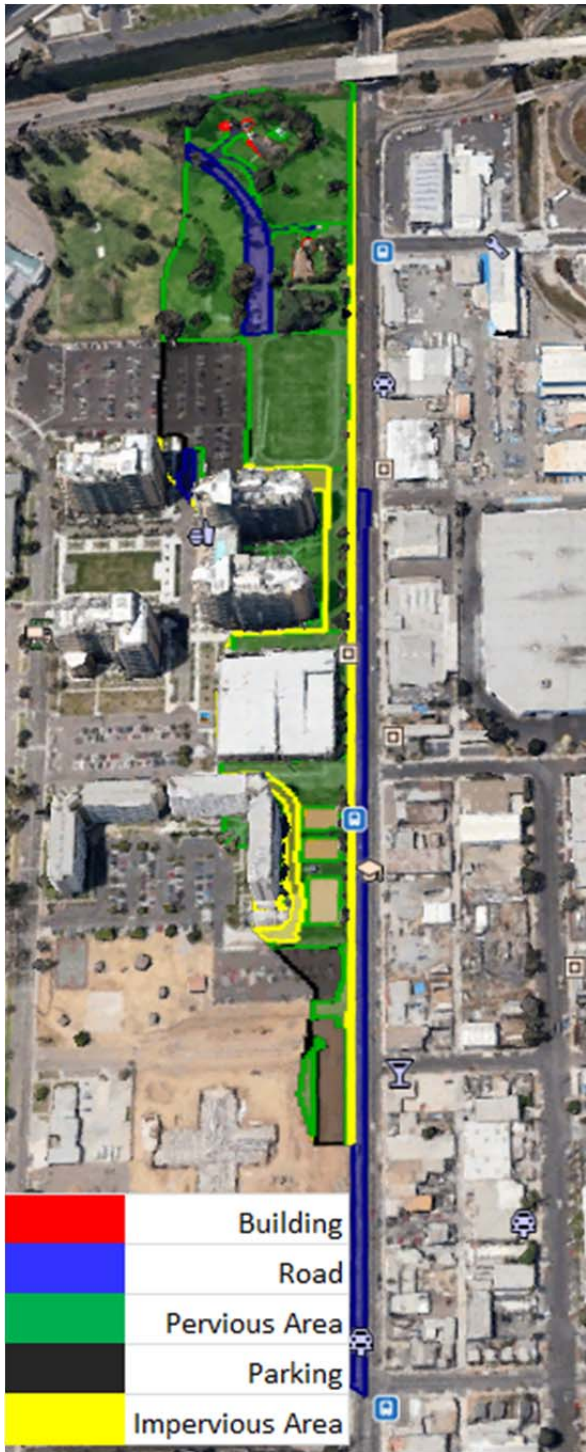
Drainage overview and Land use characterization for NBSD Outfall 51
