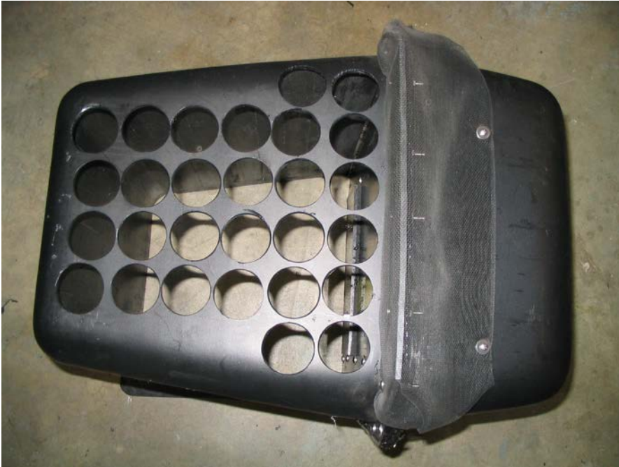
Figure 3.12: Looking at bottom of UpFlow™ filter, main inlet with large holes (but without cover screen) and weep hole tubes and finer screen at right.
