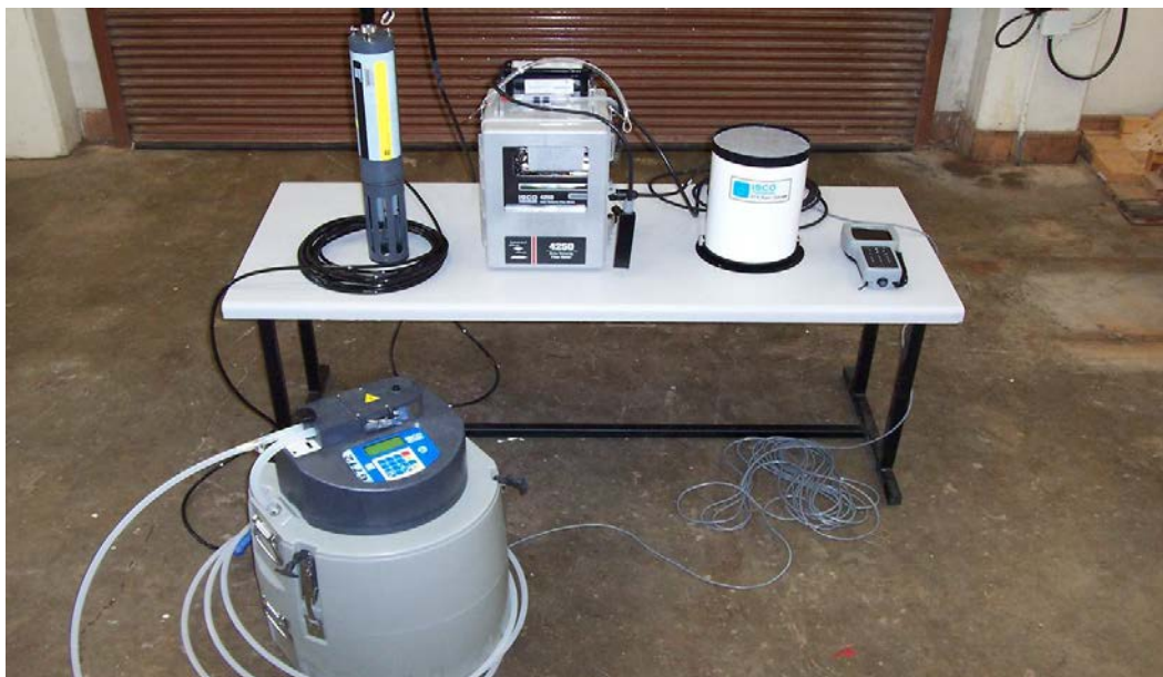
Figure 6.1: From bottom left to right 1) ISCO 6712 automatic sampler 2) YSI 6600 Sonde 3) ISCO 4250 Flow Meter 4) ISCO 674 Tipping bucket rain gauge 5) YSI Sonde data logger
