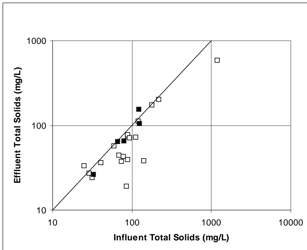
Scatterplot of observed influent and effluent total solids concentrations (filled symbols are events that had minor filter bypasses).
