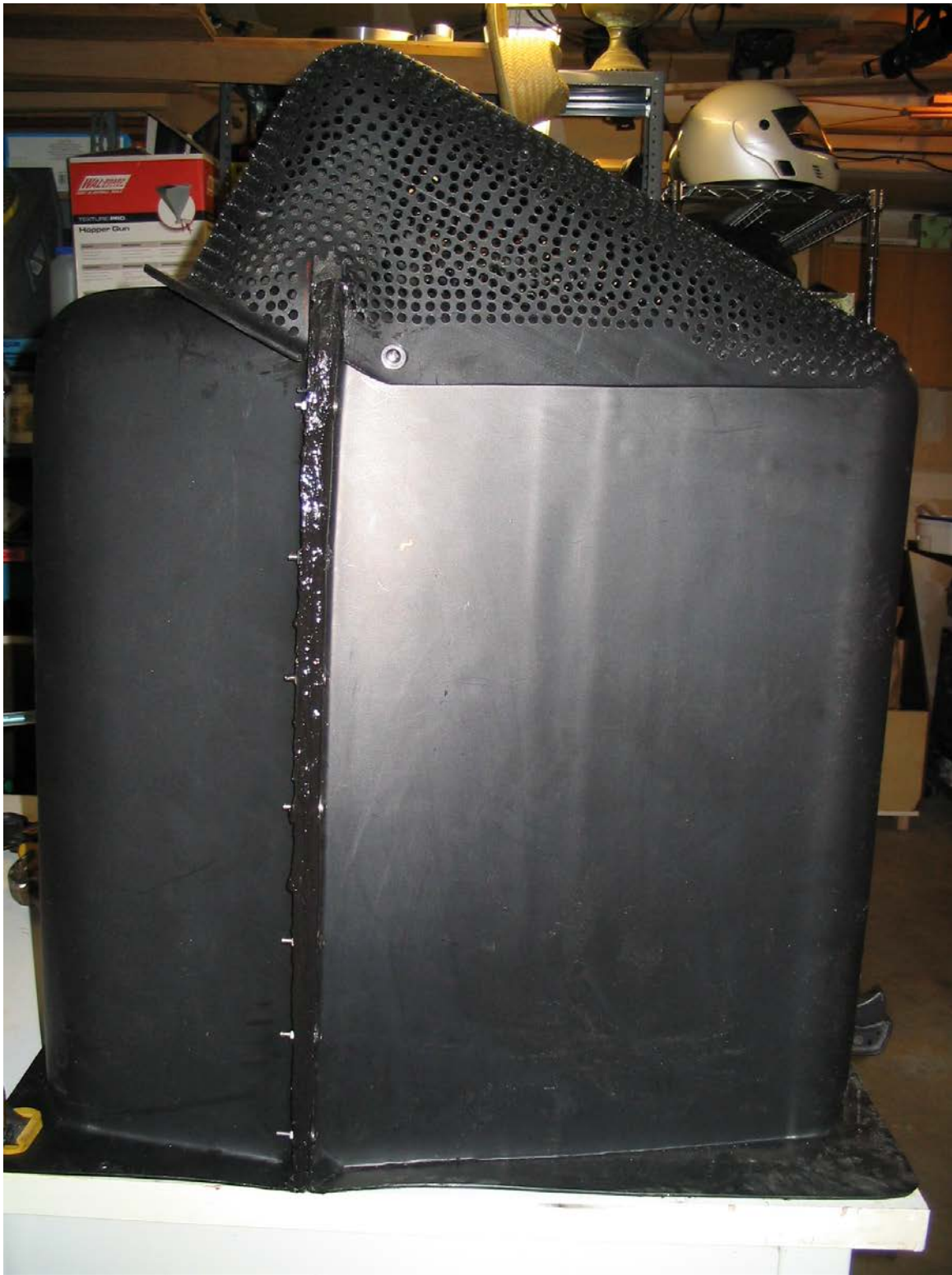
Figure 3.14: Side view of upflow chamber (upside down) with inclined floatable screen installed
