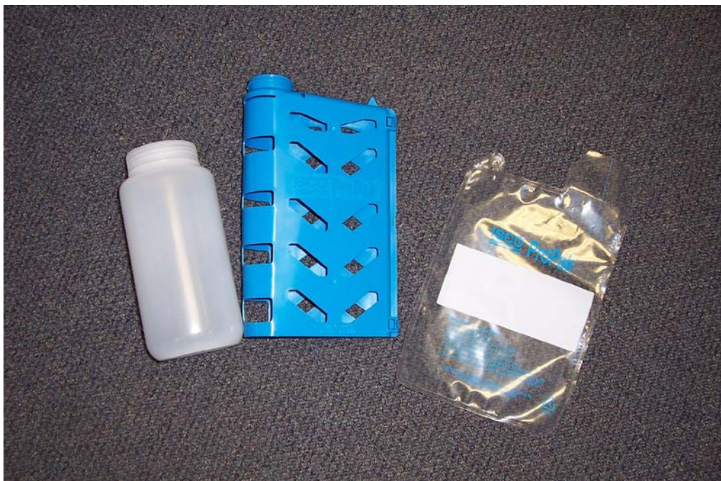
Figure 6.3: ISCO Propack, Propack holder and Nalgene bottle used to store samples
