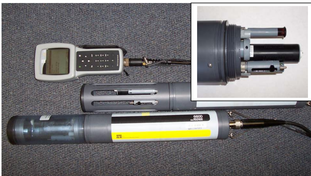
Figure 6.2: YSI 6600 sondes and data logger, Inset – Close look at the sensors
