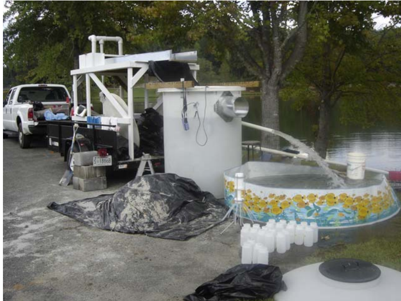
Figure 37. Full-scale physical model while performing scour tests with a sediment mixture as pre-deposited sediment material.
