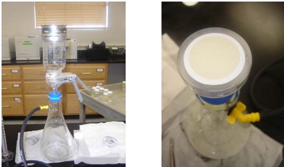
Figure 16. Procedure to determine SSC from the composite samples collected during the scour tests; sieving setup (left); a 0.45 \mu\text{m} micro-pore with sediment (right).
