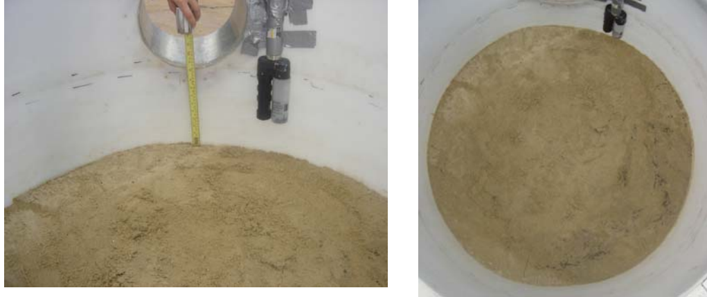
Figure 59. Placement of sediment and measurement of initial depth below the outlet.
