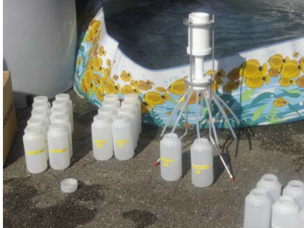
Figure 15. USGS/Decaport cone water sample splitter and 1-Liter sampling bottles.
