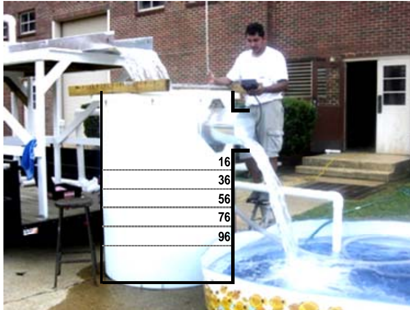
Figure 10. Full-scale physical model with the elevations for velocity measurements.
