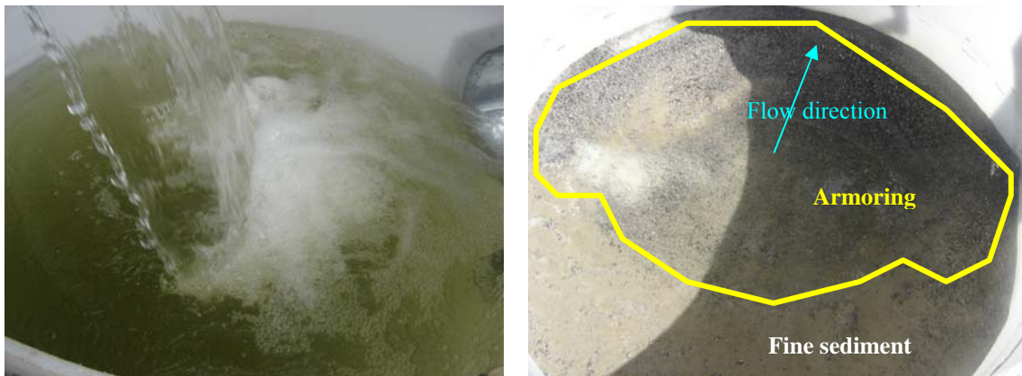
Figure 39 Armoring layer formation on sediment mixture surface. Left: Plunging water jet impacting the water surface in catchbasin sump. Right: Armoring layer.
