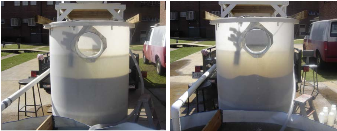
Figure 61. Initial (left) and final (right) stages of scour test with homogeneous sediment material. Test performed with sediment at 24 cm below the outlet or overlaying water depth of 24 cm.
