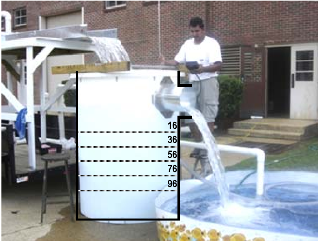
Figure A.5. Location of the five layers for velocity measuring. Depth below the outlet (cm).
