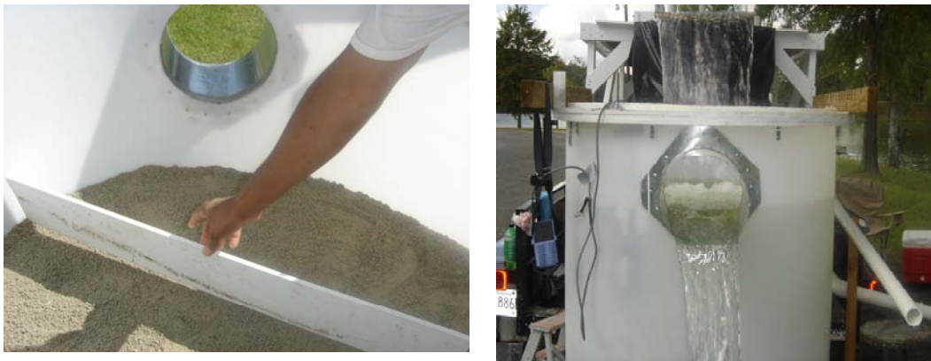
Figure 14. Placement of sediment at 25 cm below the outlet (left); performing scour test (right).
