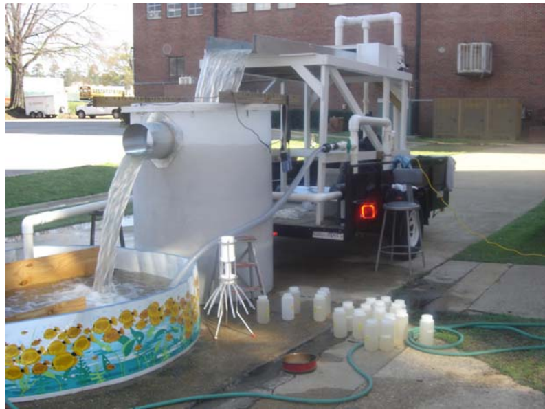
Figure 60. Full-scale physical model while performing scour tests on sediment with homogeneous particle size. See the USGS/Decaport cone water sample splitter and the 1.0 L sampling bottles.
