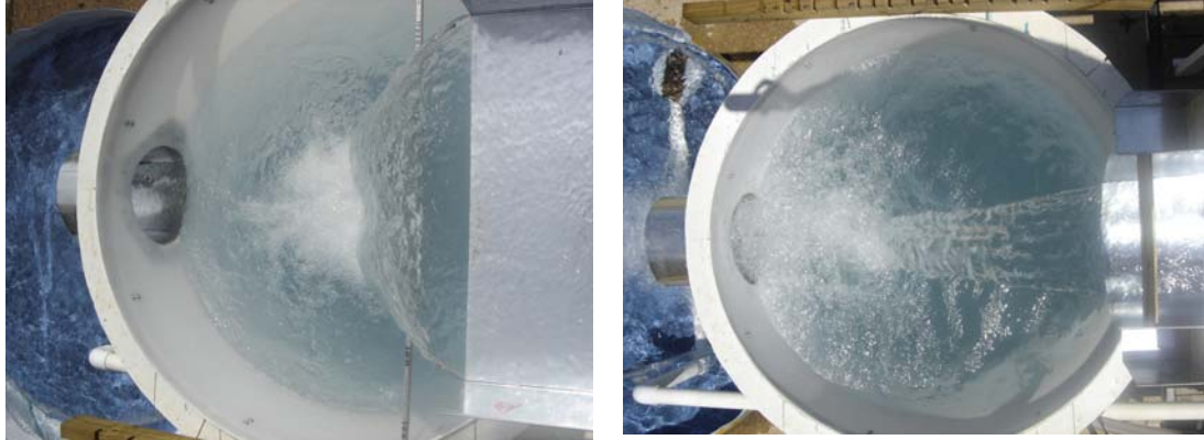
Figure 32. Top view of the full-scale physical model while performing hydrodynamic tests with the 50-cm rectangular inlet (left) and with the 300-mm pipe inlet, both at 5 L/s flow rate.
