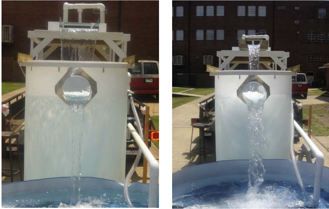
Figure 31. Front view of the full-scale physical model while performing hydrodynamic tests with the 50-cm rectangular inlet (left) and with the 300-mm pipe inlet, both at 5 L/s flow rate.
