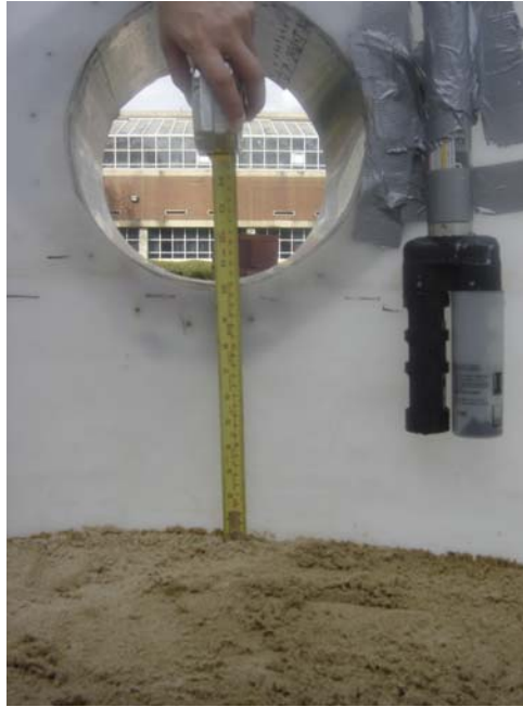
Figure 17. Location of HORIBA probe to measure turbidity next to the outlet.
