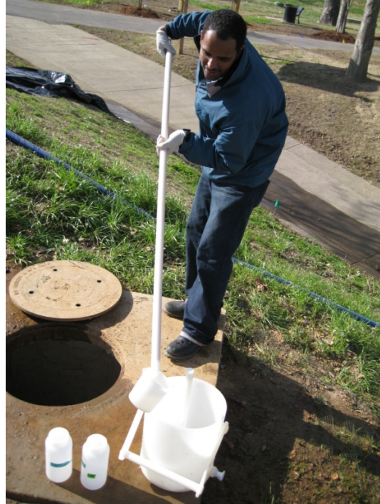
Samples are taken from the effluent box
