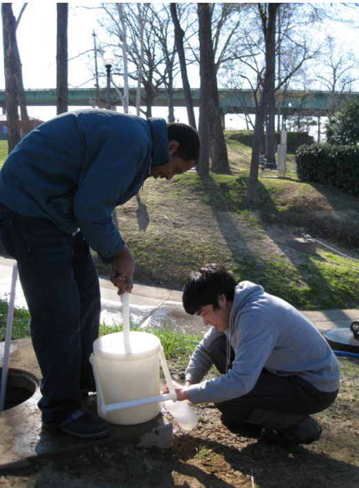
Sample splitting using churn splitter
