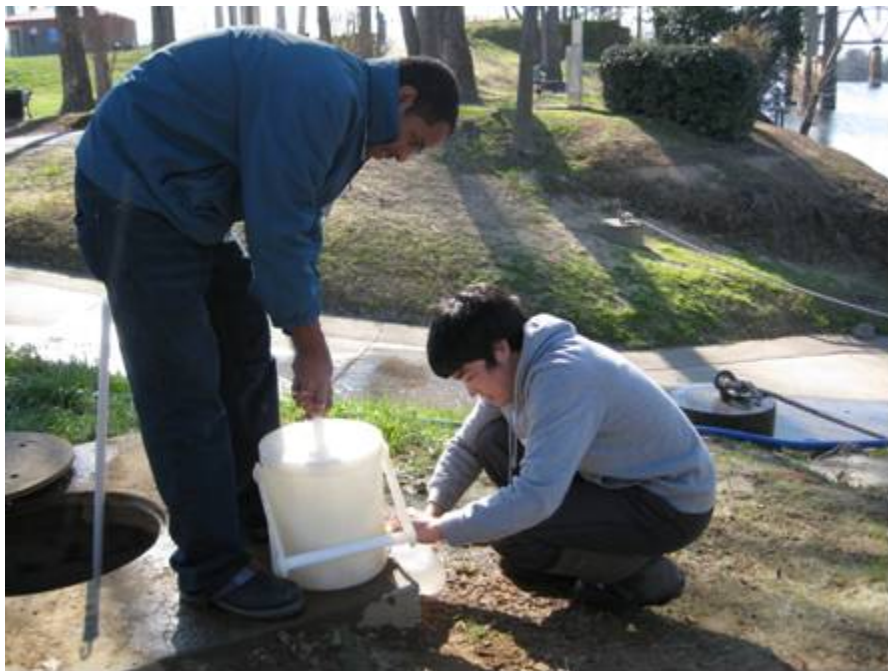
Figure 29. Sample Splitting Using Churn Splitter
