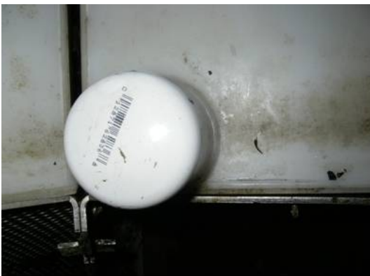
Cap installed over the draindown opening for maximum capacity determination
