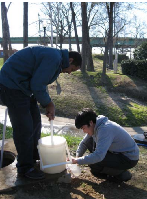
Sample splitting using churn splitter
