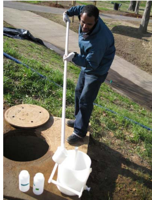
Samples are taken from the effluent box
