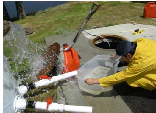
Pumped river water is discharged from splitter barrel to the 11 gallon plastic tray to manually measure the flow
