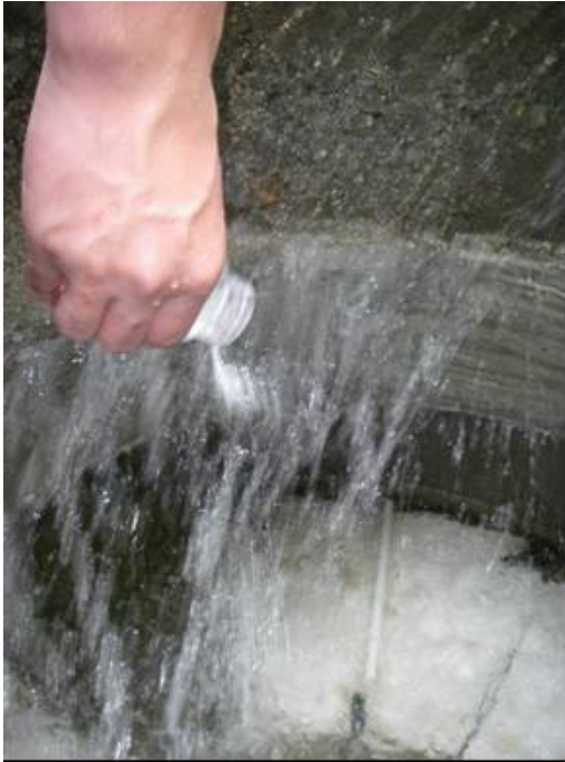
Sediment mixture is added to the flow
