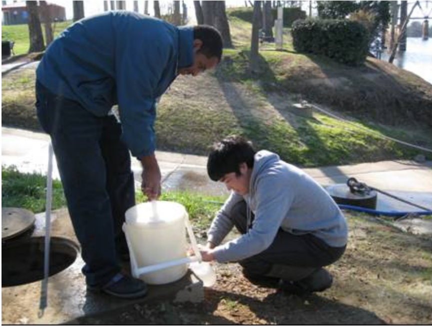
Figure 29. Sample Splitting Using Churn Splitter
