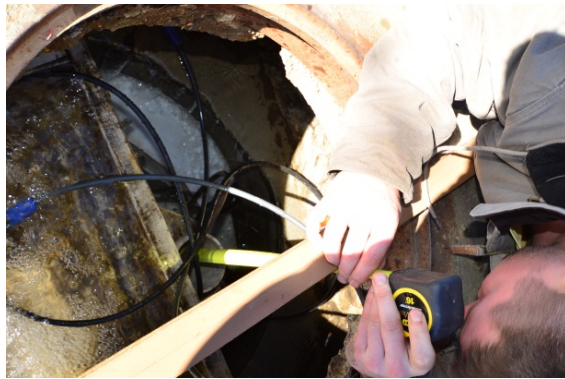
Checking stage in stilling well placed in filter chamber for comparison with continuously recording stage monitor
