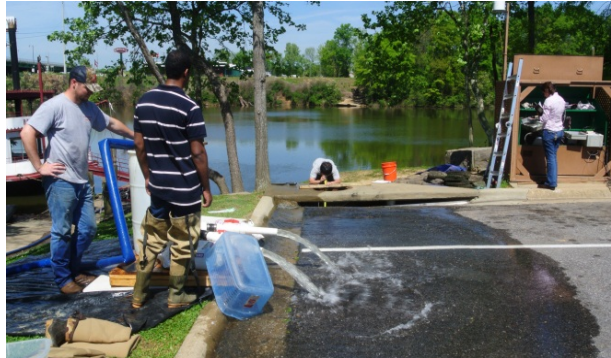
Flow tests of new media bags showing controlled flow
