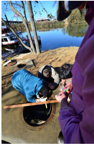
Recording water level drop after completely filling Upflow Filter
