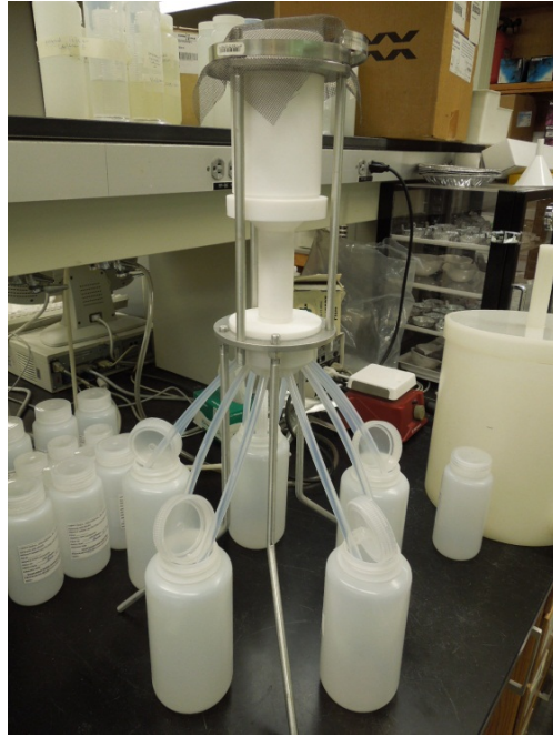
Figure 15: Cone Splitter Setup in Laboratory Sample Processing
