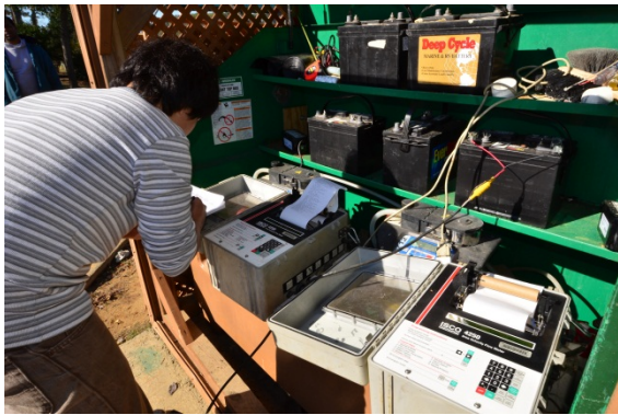
Checking outfall flow monitor (area-velocity sensor) and chamber stage monitor during calibration
