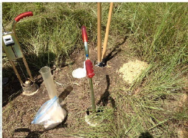
Figure 4-30 Infiltration test and soil sampling at location 5 showing typical brown colored surface soil color
