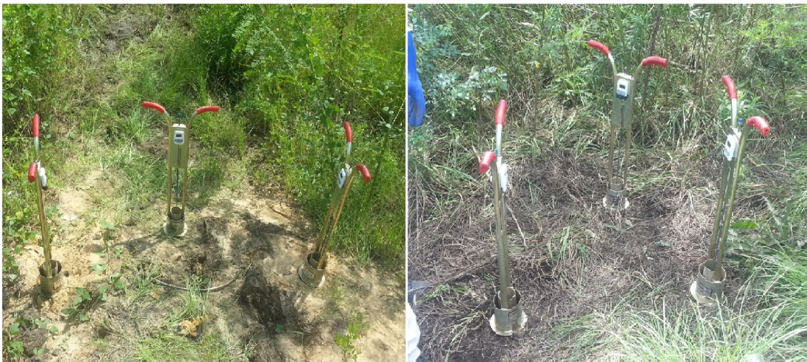
Figure 3-41 Photographs showing infiltrometer test setup
