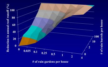
Two 35 gal. rain barrels, plus one 160 ft<sup>2</sup> rain garden, per house can reduce the total annual runoff quantity from directly connected roofs by about 90%
