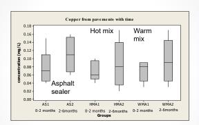
Cu release from the pavements showed a weak increasing trend with the highest concentrations being 170  $\mu g/L$ , 170  $\mu g/L$  and 160  $\mu g/L$  for the final sample at the end of 6 months of aging of the pavements.
